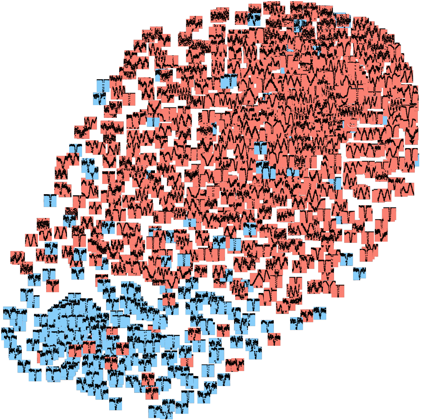
FIG. 9.— Visualizing the geometric space in which our convolutional neural network embeds its input light curves. We used the t-SNE algorithm for dimensionality reduction to create a 2-dimensional embedding such that light curves that are close in the original space are also close in the 2D space. Light curves that are far apart in 2D space are not necessarily far apart in the original space. Notice that true planet candidates (colored blue) are close to other planet candidates, and false positives (colored red) are close to similarly-shaped false positives.
