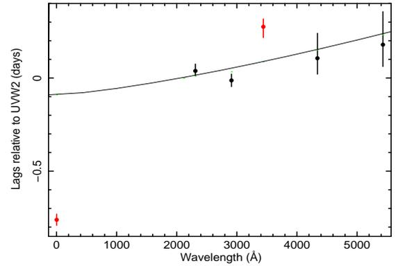
**Figure 8.** Lags relative to UVW2 derived using JAVELIN [Zu et al. \(2011, 2013\)](#). The thin line is a power law fit with index 4/3 to the model lags (shown as small green dots). Here the model lag is the time for half of the light to be received.
