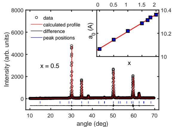
FIG. 1: (Color online) x-ray diffraction pattern for the  $x = 0.5$  composition. Peak positions are marked with small vertical bars. The line at the bottom indicates the difference between the measurement and the model prediction. Inset shows the doping dependence of the unit cell parameter  $a_0$  across the series. The straight line indicates that investigated compounds follow Vegard's law<sup>35</sup>.
