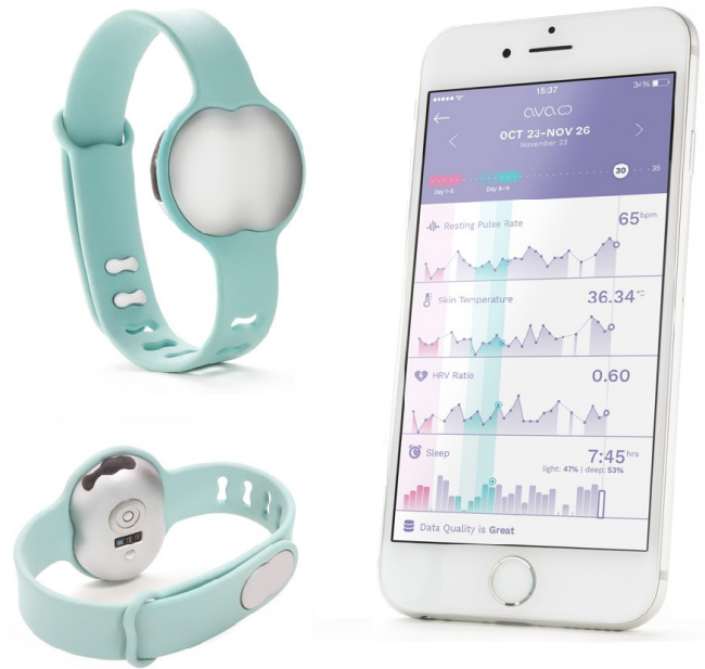
Fig. 1. Ava smart-bracelet with a multi-wavelength (green and infra-red) photoplethysmographic optical sensor.
