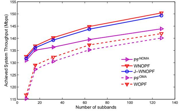
Fig. 5. Achieved system throughput vs.  $S$ , for  $K = 15$ .
