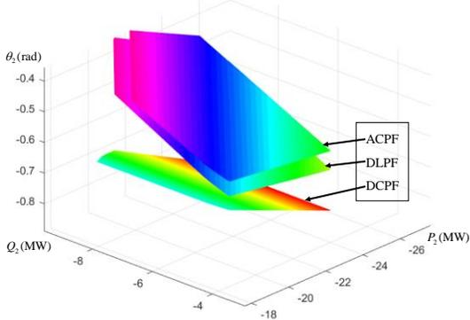
Fig. 2. Visualization of ACPF, DCPF, and DLPF in a two-bus system
