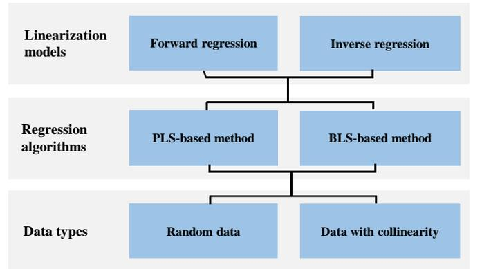
Fig. 3. Framework of data-driven power flow linearization
