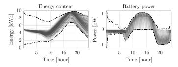
Fig. 4. Energy content and battery power for self-consumption of 500 scenarios. The dashed black lines denote the limits  $(E_{min}^{sc}, E_{max}^{sc})$  and  $(P_{min}^{sc}, P_{max}^{sc})$  from the rule-based charging policy.
