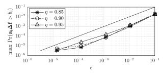
Fig. 2. Maximum probability of constraint violation with the equivalent state feedback controller (9), for various values of  $\epsilon$  and round trip efficiencies  $\eta$ , calculated with  $n_R=10^6$  samples. The solid black line denotes the maximum allowed probability.
