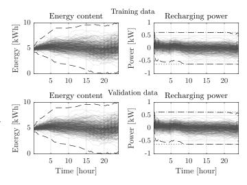
Fig. 1. Energy content and recharging power of the battery, for the frequency data in the training set (top) and the validation set (bottom), discretized according to (3) The dashed lines show the maximum and minimum cases, according to (6). The dotted lines show the maximum and minimum recharging power that is allowed, following (1e). Each line represents a frequency sample of one day.
