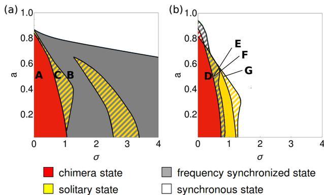
FIG. 2. Map of regimes in the parameter space of coupling strength  $\sigma$  and threshold parameter  $a$ . (a) Empirical structural connectivity,  $N = 90$ , (b) modular fractal connectivity,  $N = 125$ . Hatched regions denote multistability of dynamical states shown with corresponding colours. The letters A, B, C, D, E, F, G mark parameter values corresponding to Figs. 4(a), 5(a), 6(a), 4(e), 5(d,g), 6(d), respectively.
