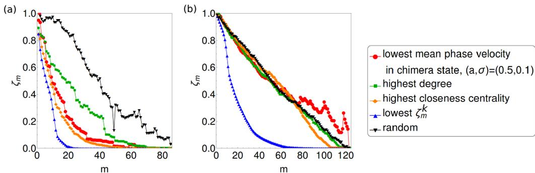
FIG. 8. Synchronizability index  $\zeta_m$  depending on the number  $m$  of progressively removed nodes. (a) Empirical structural connectivity; (b) modular fractal connectivity. All measures except the mean phase velocities are recalculated after each removal.
