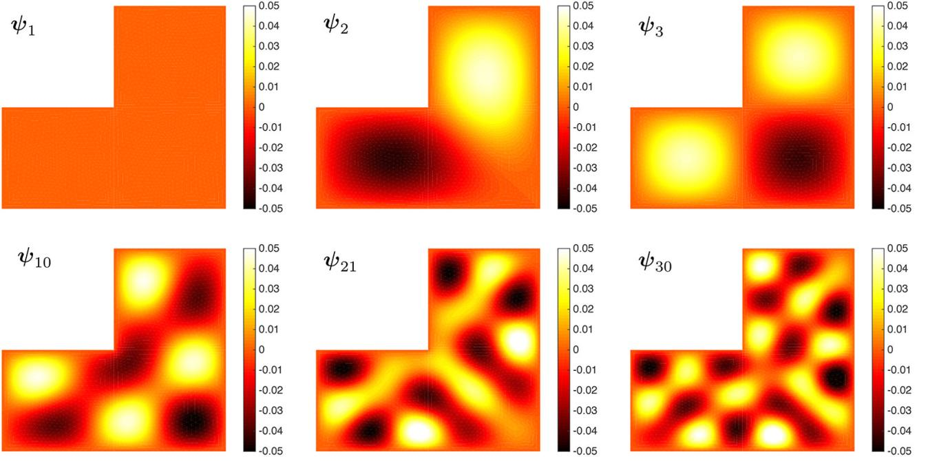
Fig. 1. First few eigenvector of the Laplacian in a L-shaped domain. The first eigenvector  $\psi_0 = 0$
