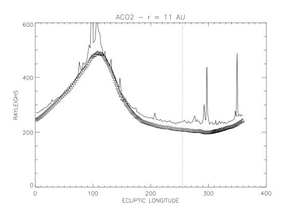
**Figure 10.** Data and model comparison for the Alice Observations of the ACO-2 Roll performed by New Horizons at 11.3 AU from the Sun. The X-axis shows the ecliptic longitude and the Yaxis is in Rayleigh. The spikes correspond to stars crossing the field of view of Alice. The data show an excess over the model in the upwind hemisphere of about 20 R, very similar to the ACO-4 roll.
