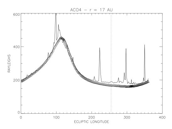
**Figure 11.** Data and model comparison for the Alice Observations of the ACO-4 Roll performed by New Horizons at 17.0 AU from the Sun. The X-axis shows the ecliptic longitude and the Yaxis is in Rayleigh. The spikes correspond to stars crossing the field of view of Alice. The data show an excess over the model in the upwind hemisphere of about 20 R, very similar to the ACO-2 roll.
