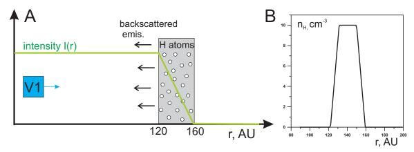
Figure 7. A. Schematic illustration of Lyman  $\alpha$  intensity backscattered at a dense layer with significantly Doppler shifted H atoms. The green solid curve shows the intensity from the layer that would be observed by spacecraft at different distances from the Sun. B. Hydrogen number density profile at the layer.
