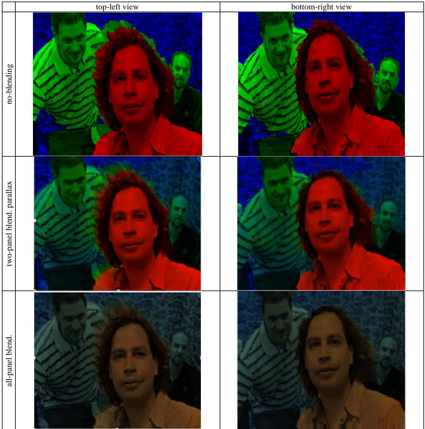
Fig. 12: Visual comparison of LF retargeting with various blending types (across rows) at two LF corner views for three-panel display. Note that the color channels are used to represent the content of the three panels with red representing the front panel, green for middle panel, and blue for back panel.
