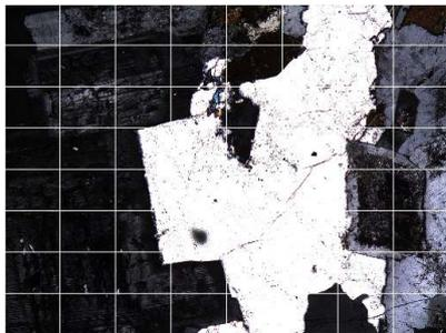
Fig. 2. An RGB image (granite) divided into 8 × 8 grid cells.
