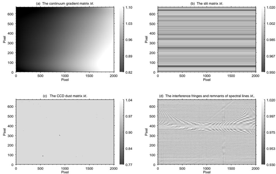
**Figure 3.** (a) The continuum gradient matrix  $M_1$ . (b) The matrix of the slit non-uniformity matrix  $M_2$ . (c) The CCD dust matrix  $M_3$ . (d) The interference fringes and remnants of spectral lines  $M_{4s}$ . The grey-scale bars give relative intensities normalized to 1.0.
