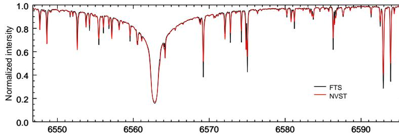
**Figure 5.** The calibration results between the NVST spectral profile (red line) and FTS spectrum (black line). The NVST spectral profile is the average of the reduced  $F_{\text{mean}}$  along the  $Y$ -direction. The  $Y$  axes gives relative intensities normalized to 1.0.
