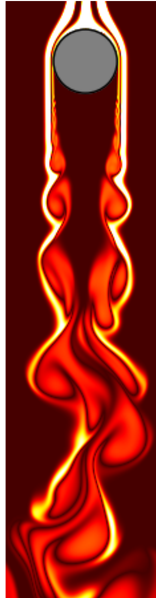
FIG. 1.—: Flow past a cylinder computed with an implementation of Stam’s Stable Fluids algorithm after \sim 3 vertical fluid crossing times on a 500 \times 2000 zone grid. Color corresponds to the density (or concentration, given that \vec{\nabla} \cdot \mathbf{v} = 0 ) of passively advected dye that is injected into the flow upstream of the cylinder. Despite using first-order differencing, the implementation is able to produce visually realistic results by diverting fluid compression into eddying motions.
