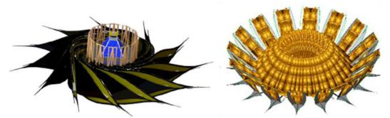
Figure 2: Starshade deployment schemes. The right panel shows the "telescoping boom" approach<sup>36</sup> and the left panel shows the "petal unfurling/perimeter truss" method<sup>35</sup> (Image credit: JPL/Caltech (left), NGAS (right).
