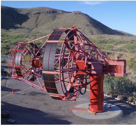
Figure 5: Prototype SCT, as of June 2017, showing both the primary and secondary baffles already installed.
