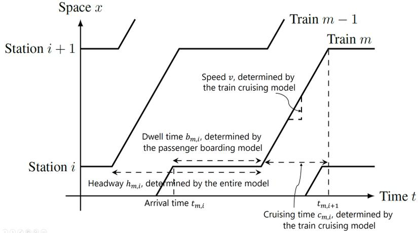
**Figure 2:** Illustration of the microscopic model of rail transit system.
