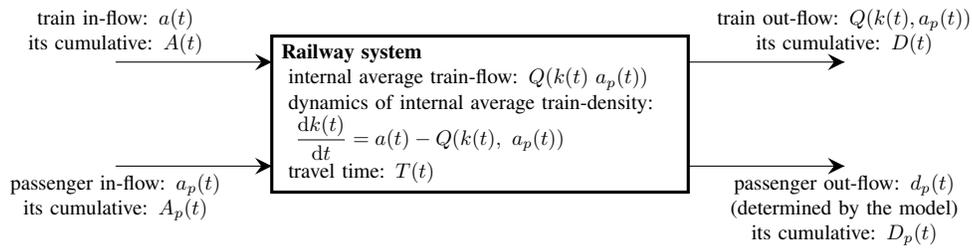
**Figure 5:** Railway system as an input–output system.
