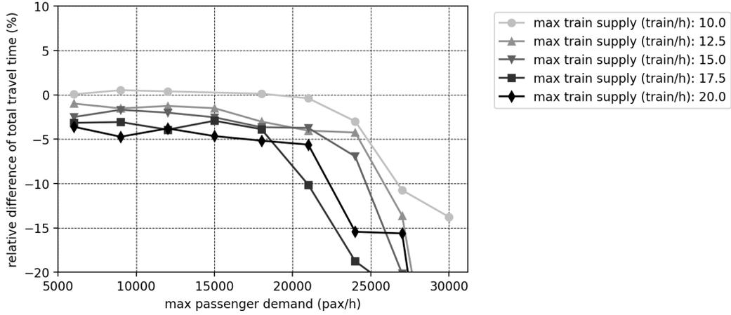
**Figure 9:** Comparison between the microscopic and macroscopic models under different demand/supply conditions.
