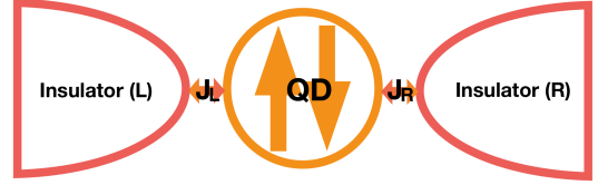
FIG. 1: Schematic representation of the system considered in this paper. A single-level quantum dot (QD) occupied by either spin \uparrow or spin \downarrow electron is coupled to two magnetic insulators (L,R). The insulating leads are also referred to as magnonic reservoirs. The corresponding coupling strengths are J_L and J_R .
