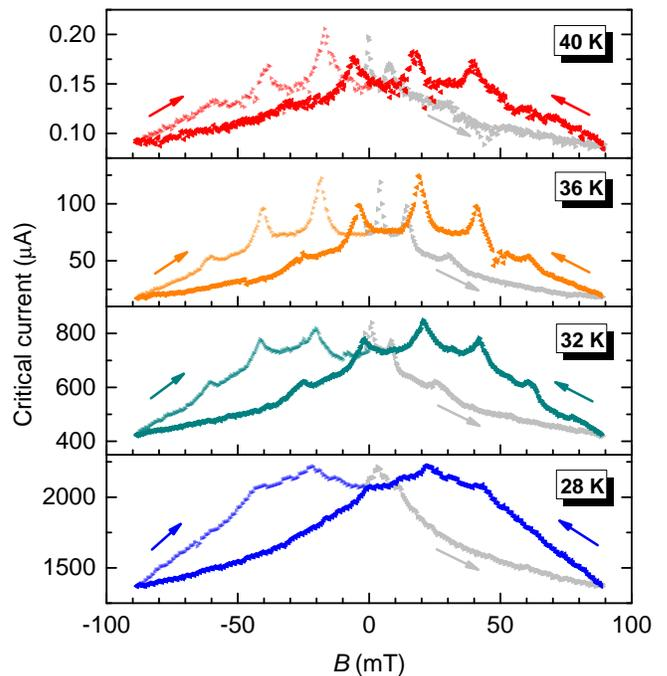
FIG. 3. Hysteretic behavior of the critical current after zero-field cooling at the respective temperature and ramping the applied magnetic field  $B$  through a full cycle. Grey symbols denote the virgin curve.
