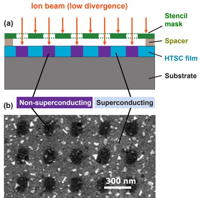
FIG. 1. (a) The principle of masked ion beam direct structuring (MIBS). (b) Scanning electron microscopy (secondary electron detection) picture of the surface of a thin YBCO film after MIBS with 75 keV  $\text{He}^+$  ion irradiation. The dark regions correspond to an array of defect-rich, non-superconducting nano-cylinders.
