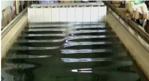
FIG. 6: (Color online) Photographic image taken at a distance of 10 m from the wave maker for a = 0.02 m, \kappa = 7.3 m ^{-1} , \chi = 0 , \theta = 0 and \gamma = 0.4\pi .
