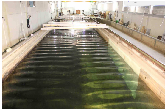
FIG. 3: (Color online) Photographic image taken at a distance of 35 m from the wave maker for the experiment presented in the top panel of Fig. 2: a = 0.01 m, \kappa = 10.8 m -1 .
