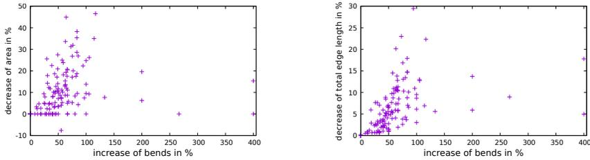
**Fig. 13.** Relation between additional bends and improvement of area and total edge length for the quasi trees
