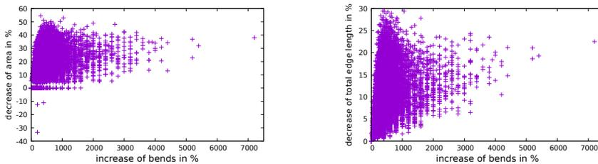
**Fig. 14.** Relation between additional bends and improvement of area and total edge length for the Rome graphs
