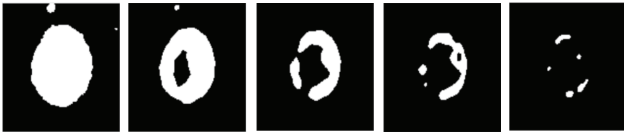
Fig. 2.— Dynamic thresholding binary maps. The Images show binary maps with thresholds of 20 (left), 44, 83, 99, and 115. The figure shows that when using a graylevel of 44 the ring is identified in the binary mask, while other graylevel thresholds show no ring.
