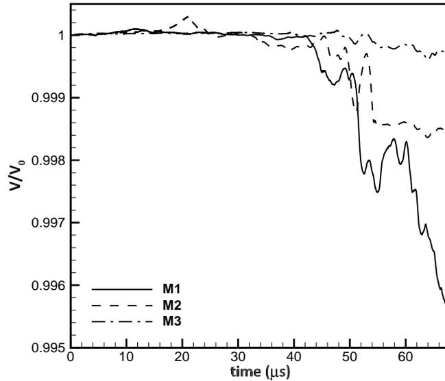
FIGURE 4. Mass conservation check for different mesh resolutions.
