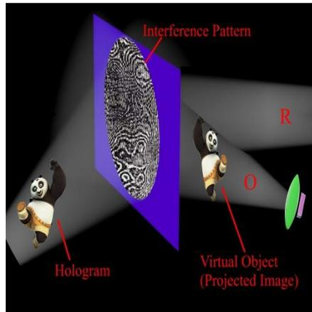
Fig. 3. The configuration of the proposed field reconstruction of holograms method. It contains an OSA (the pink component at right side), an imaging lens (the green component at right side), a screen (the blue square in the middle), a reference light source and an eye tracking component (not shown in the picture).
