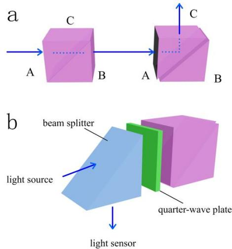
Fig. 1. Illustration of basic function of TOS. a) Two TOS in series b) a TOS connected with a quarter wave plate followed by a polarization beam splitter
