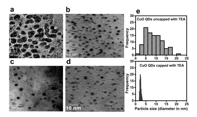
**Figure 3**. TEM images of (a) uncapped copper oxide QDs and (b) capped copper oxide QDs (c) TEM images of digestively ripened copper oxide QDs that are 120 days old. It may be noted from (a) that without capping particle coalescence is a concern. (d) TEM images of digestively ripened copper oxide QDs that are 1 year old. (e) Shows particle size distribution of copper oxide QD before and after digestive ripening.
