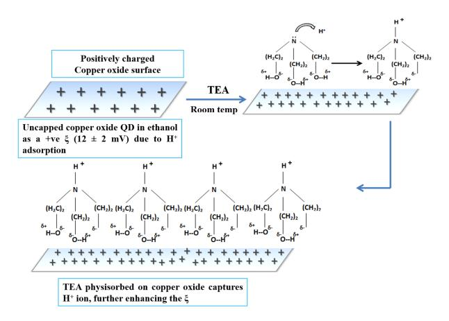
Figure S1. Proposed mechanism for the observed increase in  $\xi$  of capped copper oxide QDs (when compared to uncapped copper oxide QDs).
