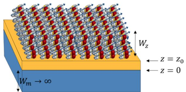
FIG. 2. *Plexciton setup.* The model consists of a surface-plasmon (SP) metal layer whose width  $W_m$  can be considered infinite in comparison with the relevant length scales of the structure. The thiacyanine molecular ensemble is separated from the metallic surface by a spacer of width  $z_0$ ; the balls and sticks represent the molecules, while the arrows denote their transition dipole moments. The molecular layer has a height  $W_z$  and is extended along the  $x$  and  $y$  planes.
