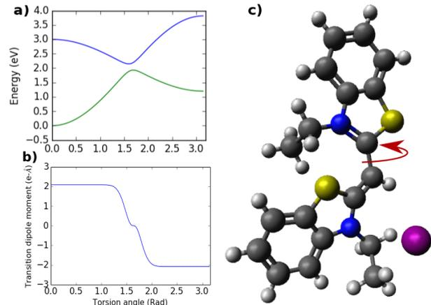
FIG. 1. a) Adiabatic potential energy surfaces (PESs) of the ground and first excited electronic states of the thiocyanine-like model molecule. b) Transition dipole moment ( $\mu(R)$ ) of the model molecule in the adiabatic basis. c) Thiocyanine molecule. There exist two geometrical isomers of the molecule, a cis- and a trans-like configuration. The cis-trans isomerization of thiocyanine-like molecules occurs via a photo-induced torsion along the bridge which connects the aromatic rings.
