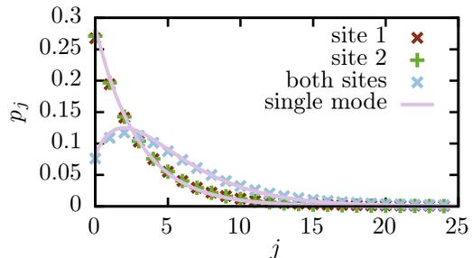
Figure 3. The probabilities of finding  $j$  particles at site 1, site 2 and at both sites obtained via the iterative approach (data points) are in very good agreement with the probabilities of the analytically solvable single-mode approach (solid lines) given by Eq. (35) and Eq. (37), respectively. The parameters used are  $N_0 = 5$ ,  $g = 0.5$  and  $\gamma = 0.5$ .
