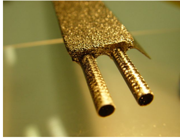
Figure 36: Photograph of a prototype mechanical support built with braided carbon pipes, embedded in carbon foam.
