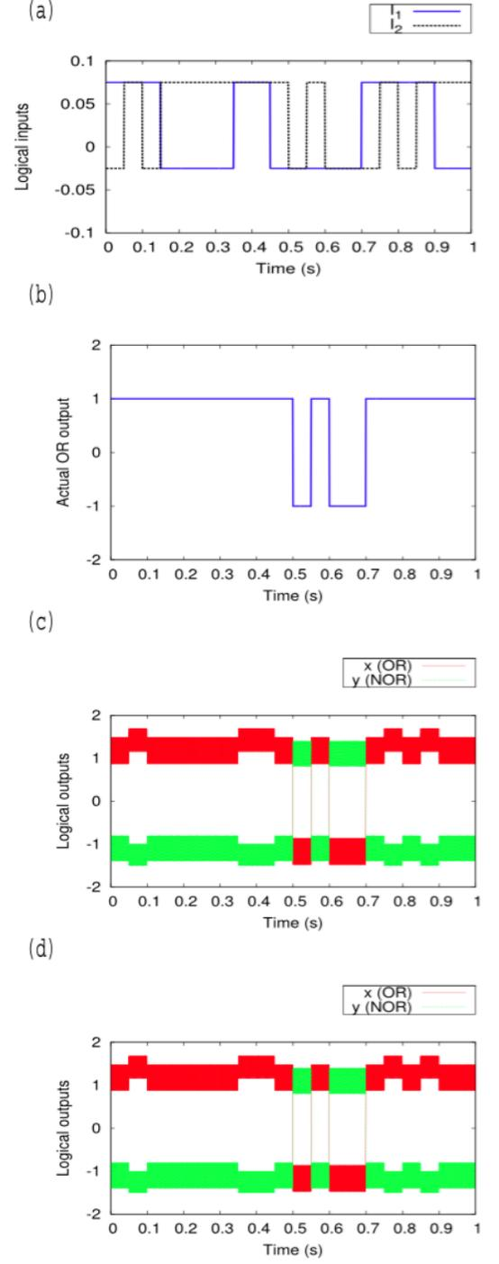
FIG. 6. Same as in Fig. 5 but with the random inputs for OR gate operation. During the interval  $[0 : 1.0 \text{ s}]$ , the state variable x mimics OR operation and the variable y mimics NOR operation.
