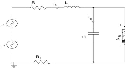
FIG. 1. Circuit realization of Murali-Lakshmanan-Chua circuit with quasiperiodically driving force.
