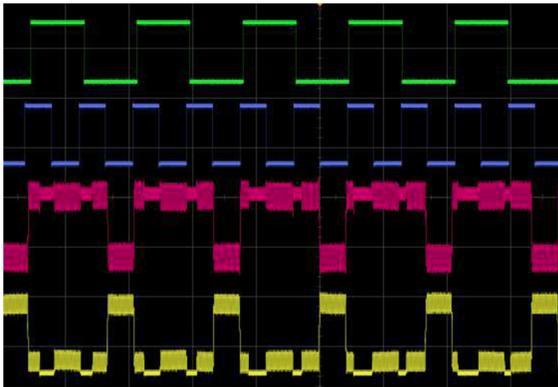
FIG. 8. Experimental confirmation of logic OR/NOR gate. From top to bottom: Green and blue square waves represent the two input signals, pink waveform represents the voltage response ( $v$ ) of QPDMLC circuit across the capacitor  $C$ , which mimics OR operation and the yellow waveform represents the voltage response ( $v_s$ ) of QPDMLC circuit across the sensing resistor  $R_s$ , which mimics NOR operation.
