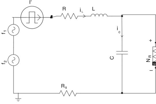
FIG. 2. Murali-Lakshmanan-Chua circuit with a second harmonic driving force  $f_2$ , having an incommensurate frequency, and random pulsed voltage source ( $I'$ ).
