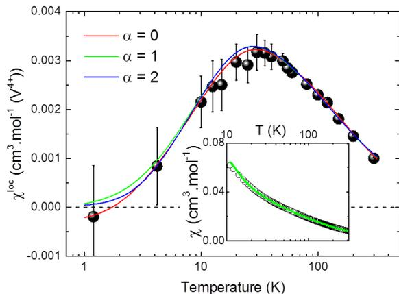
Figure 3. Local NMR susceptibility of the kagome layers  $\chi^{loc}$ . The lines are fits to  $A\chi_{kago}^{th} + C$  (see text). Inset: SQUID macroscopic susceptibility (circles) and fit to a combination of  $\chi_{kago}^{th}$  ( $\alpha = 1$ ) and a paramagnetic contribution from the  $V^{3+}$  (line) [24].
