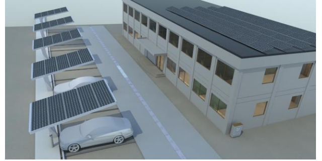
Fig. 1. Design of solar powered EV charging station
