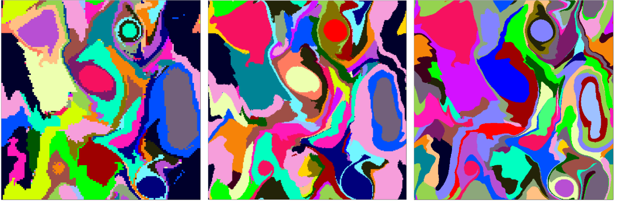
FIG. 10. Hierarchical transfer operator method with 128 (left), 256 (middle) and 512 (right) boxes. For all cases: Each box contains 16 points; 8 levels of hierarchy where used; and \mu -tolerance is set to 5 \times 10^{-2} .
