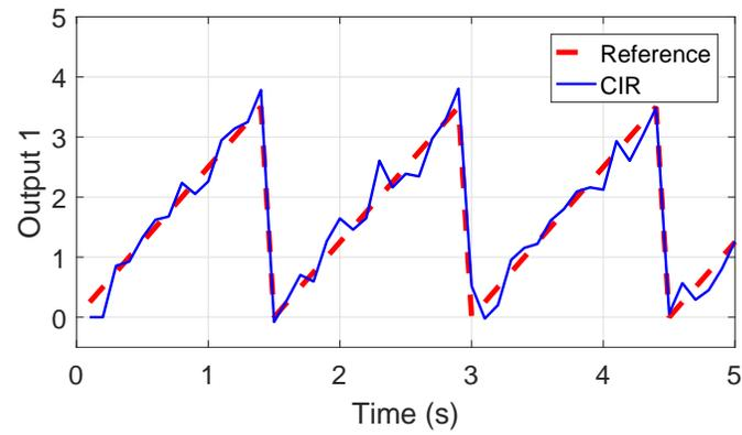
Figure 9: Commands can be accurately followed for a system with  $l > p$  if  $p - l$  outputs are ignored keeping  $\text{rank}(CB) = l$ .
