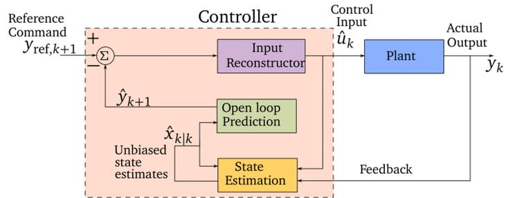
Figure 1: Schematic of command following controller.
