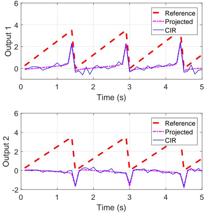
Figure 8: System outputs can track the projections of the reference command on  $\mathcal{R}(M_r)$
