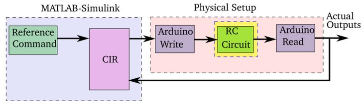
Figure 5: Setup for real time command following using CIR
