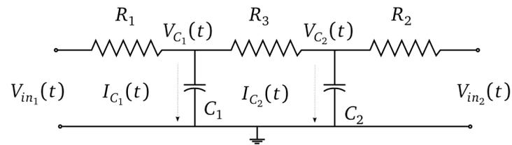
Figure 6: A second order MIMO RC circuit
