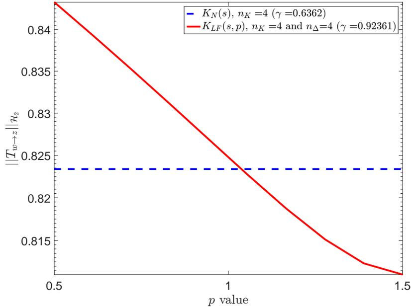
Figure 4:  $\mathcal{H}_2$  performance evaluation function of the  $\mathbf{p}$  tuning parameter. Red solid line: looped systems with  $\mathbf{K}_{LF}(s, \mathbf{p})$ , and dashed blue for  $\mathbf{K}_N(s)$ .
