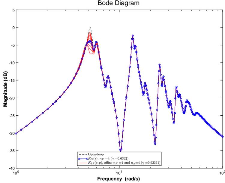
Figure 3: Bode diagram of the open-loop (dashed black), the closed-loop obtained with the nominal control  $\mathbf{K}_N(s)$  (obtained for  $\mathbf{p} = 1$ , blue rounded), and the parametric controller  $\mathbf{K}_{LF}(s, \mathbf{p})$  (solid red lines).
