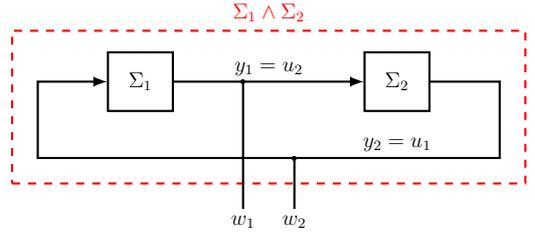
Fig. 3. Interconnection of LTI stochastic processes  $\Sigma_1$  and  $\Sigma_2$  of Example 10 in an input-output representation.
