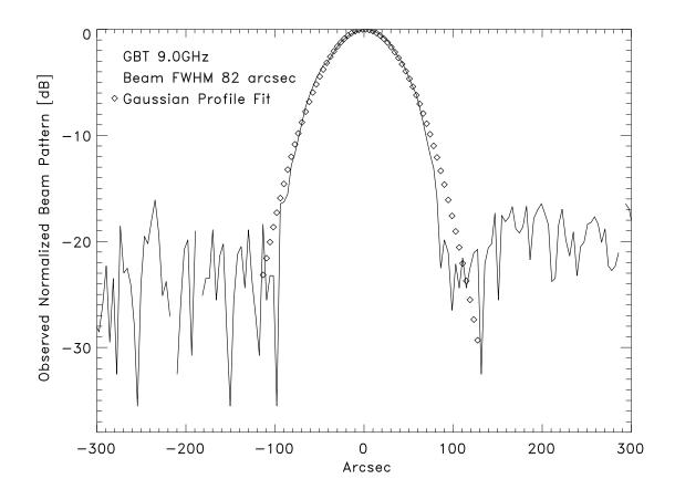
Figure 1: The normalized GBT beam profile in dB observed at 9.0 GHz shown as the solid line as a function of arcsec from 0510+1800 along the elevation axis. The diamonds show a Gaussian fit to the observed profile. The absolute value of the data was used for plotting on a logarithmic scale to show the relative noise level of the observations (-20dB).
