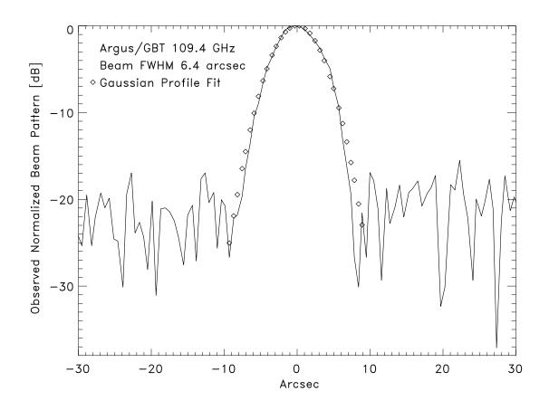
Figure 2: The normalized GBT beam profile in dB observed at 109.4 GHz shown as the solid line as a function of arcsec from 3C273 along the elevation axis. The diamonds show a Gaussian fit to the observed profile. The observed beam of 6.4 arcsec is the smallest beam observed to date with the GBT.
