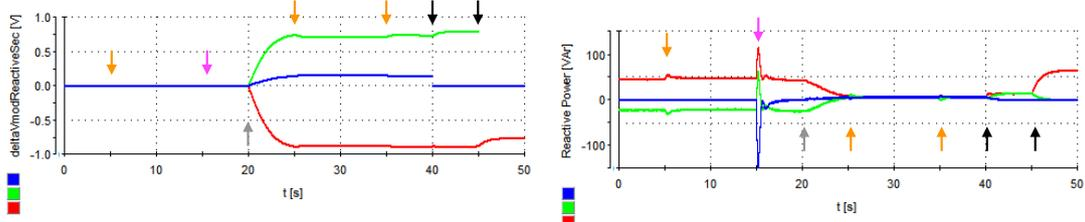
(a) Amplitude deviations  $\Delta V_i^Q$  in (17) leading to the sharing of total reactive power.
