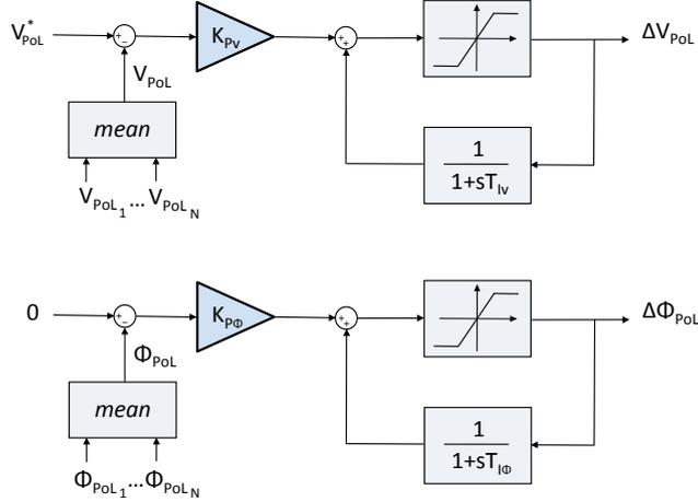
Figure 6: Coordinated control layer: computation of correction terms  $\Delta V_{PoL}$  and  $\Delta \phi_{PoL}$ . Parameters  $K_{PV}$  and  $K_{P\phi}$  are the voltage and phase proportional coefficients, while  $T_{IV}$  and  $T_{I\phi}$  are the voltage and phase integral time constants.
