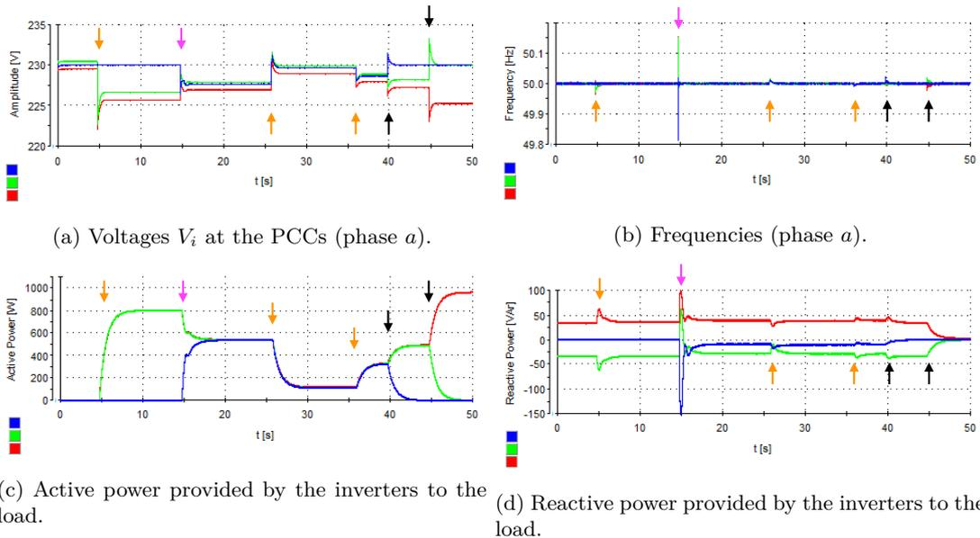
Figure 10: Voltage regulation at the PCCs with resistive load (Section 5.2.1). Red, green and blue lines are, respectively, for VSC 1, 2 and 3. Load change, plug-in and unplugging events are indicated with orange, magenta and black arrows, respectively.
