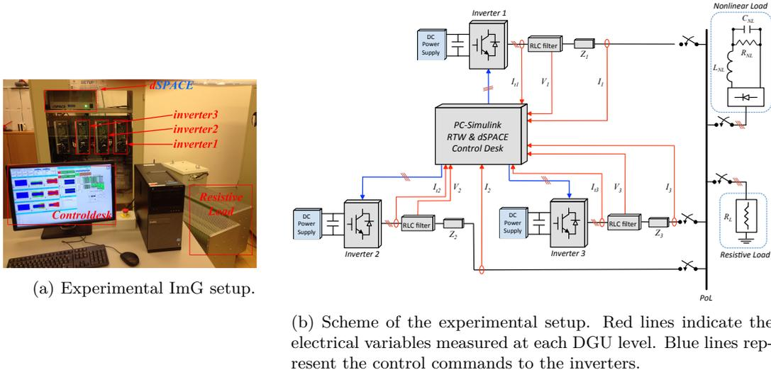
Figure 9: Experimental validation: ImG setup and implemented control scheme.
