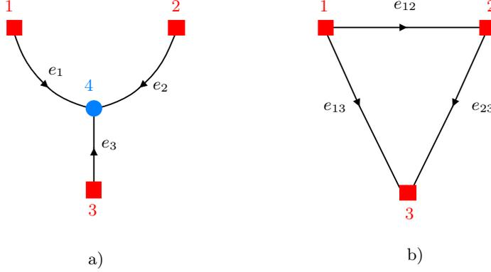
Figure 2: Graphs of a bus-connected ImG with 3 DGUs (on the left) and its equivalent load-connected network (on the right). Red squares indicate DGUs with corresponding local loads  $I_{L_i}$  (boundary nodes), while the blue circle denotes the unique load at the common bus (internal node).
