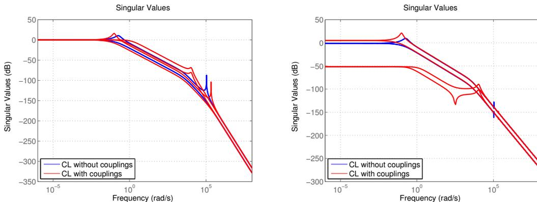
(a) Singular values of the transfer function matrix from  $dq$  voltage references to  $dq$  voltages at the PCCs. (b) Singular values of the transfer function matrix from  $dq$  voltage references to  $dq$  currents in the filters.
