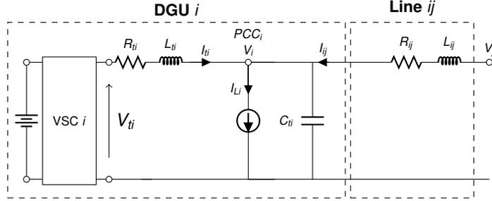
Figure 1: Equivalent single-phase electrical scheme of DGU  $i$  and power line  $ij$  in a load-connected ImG.
