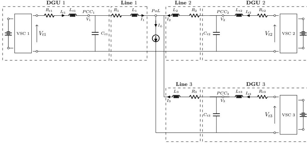
Figure 3: Electrical scheme of a bus-connected ImG composed of three DGUs and a common unmodeled load.
