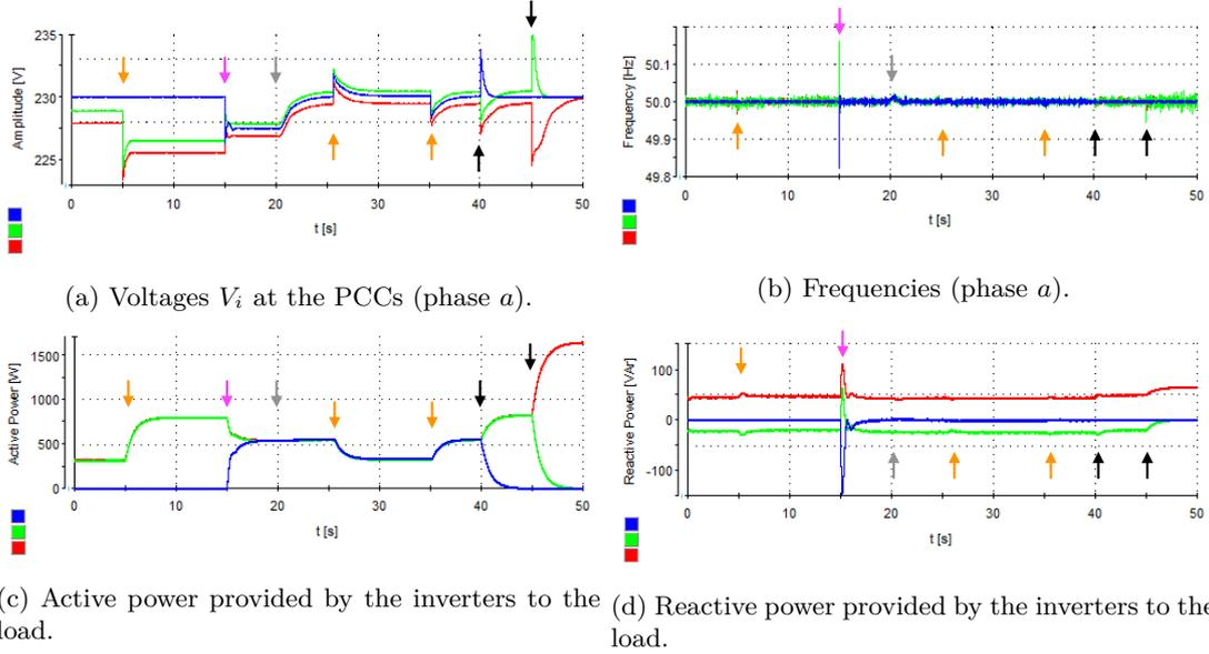
Figure 13: PnP regulators and coordinated controllers for voltage tracking at the PoL with nonlinear load. Red, green and blue lines are, respectively, for VSC 1, 2 and 3. Load change, plug-in and unplugging events are indicated with orange, magenta and black arrows, respectively. Moreover, the grey arrow denotes the activation of secondary controllers described in Section 4.1.
