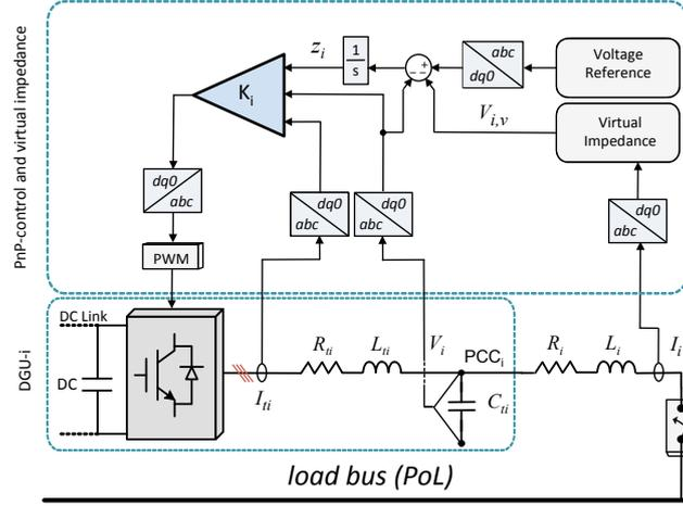
Figure 4: Bus-connected DGU equipped with local PnP regulator and virtual impedance loop.
