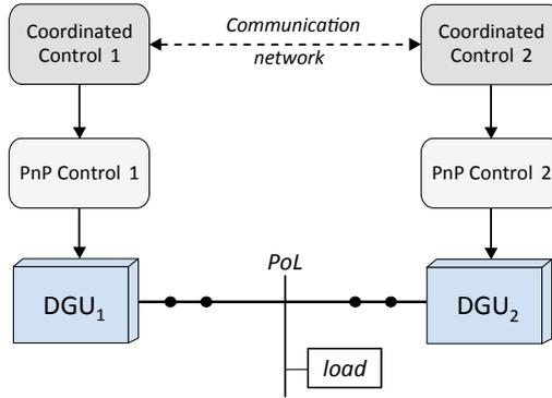
Figure 7: Scheme of the coordinated control.
