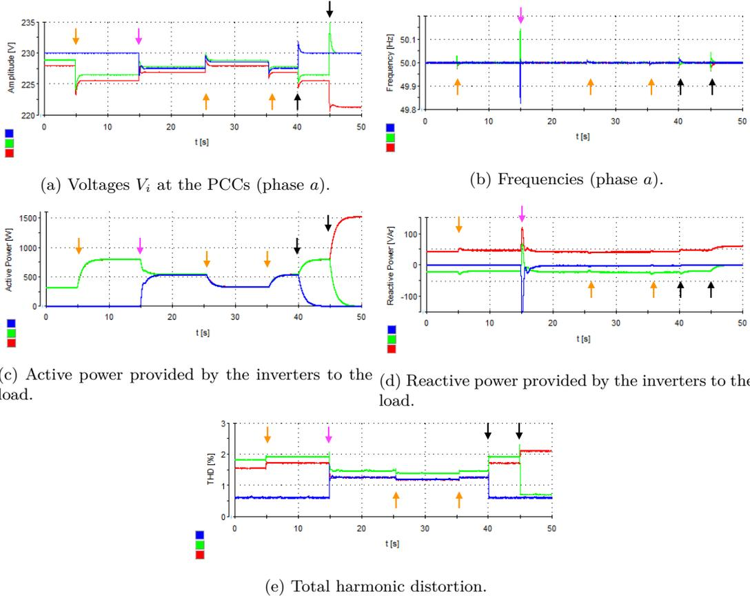
Figure 12: Voltage regulation at the PCCs with nonlinear load (Section 5.2.3). Red, green and blue lines are, respectively, for VSC 1, 2 and 3. Load change, plug-in and unplugging events are indicated with orange, magenta and black arrows, respectively.
