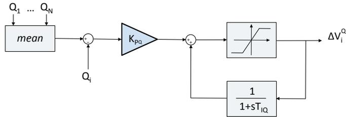
Figure 8: Control scheme for the computation of  $\Delta V_i^Q$ . Parameters  $K_{PQ}$  and  $T_{IQ}$  are the reactive power proportional term and the reactive power time constant, respectively.
