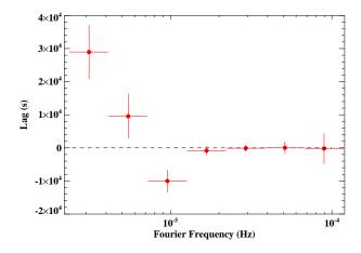
**Figure 5.** The lag-frequency spectrum computed using ~ 770 ks of *Suzaku* data. The lag is calculated between the soft (0.3-0.8 keV; 0.36-0.95 keV) in the rest frame) and the hard (1-3 keV; 1.18-3.55 keV) in the rest frame) energy bands, and a negative lag means that the soft band lags behind the hard band. It can be seen that the most negative lag is  $10000 \pm 3400 \text{ s}$  at  $9.58 \times 10^{-6} \text{ Hz}$ .
