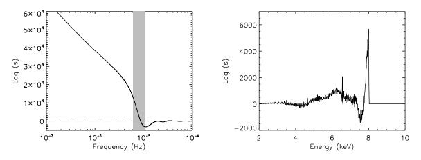
**Figure 9.** Left: The lag-frequency spectrum for the energy-averaged iron line, assuming  $i = 65^\circ$ ,  $h = 10 \ GM/c^2$ , a = 0.998 and  $\log M = 8.91$ . The grey shaded region shows the frequency range where the soft lag is detected in PDS 456, and over which the lag-energy spectrum (right-panel) is calculated. *Right:* The lag-energy spectrum over the frequency-range  $[7.2 - 12.7] \times 10^{-6}$  Hz, assuming a reflection fraction of 0.6, and parameters listed previously.
