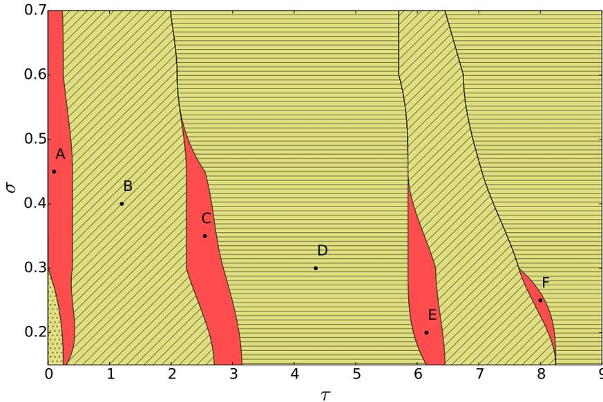
**Fig. 2.** (Color online) Chimera tongues (red), in-phase synchronization (horizontally striped yellow region) and coherent traveling waves (diagonally striped yellow region) in the parameter plane  $(\tau, \sigma)$  for  $b_{init} = (11011)$ ,  $n = 4$ ,  $N = 626$ ,  $\varepsilon = 0.1$ . At the transition to a chimera region we can observe chaos (dotted yellow region at small  $\tau, \sigma$ ).
