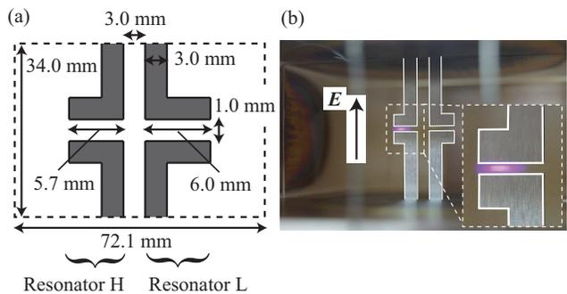
FIG. 1. (a) Unit structure of the EIT-like metasurface. The metasurface is made of aluminum with a thickness of 1.0 mm. (b) Photograph of the metasurface when microplasma is generated in the gap of resonator H. The outline of the structure is marked by white solid lines. The inset shows the magnification of the gap of resonator H.
