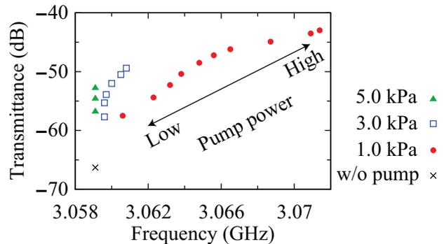
FIG. 6. Relationship between the center frequency of the higher-frequency transmission dip and the transmittance at that frequency for  $p_{\text{air}} = 1.0$  kPa, 3.0 kPa, and 5.0 kPa. The data points correspond to those in Fig. 8; see Fig. 8 for the pump power at each point.
