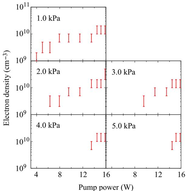
FIG. 8. Electron density plotted against pump power for  $p_{\text{air}}$  values ranging from 1.0 kPa to 5.0 kPa. The electron density was estimated to be in the range represented by the bars. The data points for  $p_{\text{air}} = 1.0 \text{ kPa}$ , 3.0 kPa, and 5.0 kPa correspond to those in Fig. 6.
