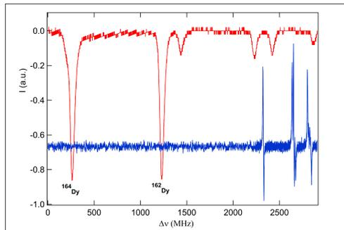
**Fig. 2.** Fluorescence spectrum (upper red curve) of the Dy atomic beam and error signal (lower blue curve) of the saturated absorption of Iodine as a function of the laser frequency near 626 nm. The largest peaks from the left come from the two bosonic species  $^{164}\text{Dy}$  and  $^{162}\text{Dy}$ , while the smaller ones belong to the fermions. We lock the laser to the left-most line of Iodine in the figure.
