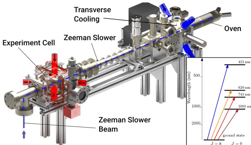
**Fig. 1.** Sketch of the experimental apparatus. Laser beams are indicated by blue (421 nm) and red (626 nm) arrows. In the inset, the  $J \rightarrow J + 1$  transitions from Dy ground state are shown. The two transitions at 421 nm and 626 nm are used for slowing and trapping, respectively.
