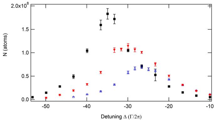
**Fig. 4.** Number of atoms in the MOT as function of the detuning in the loading phase respectively with: (full squares) 2.0 MHz laser linewidth, (full triangles) 1.1 MHz laser linewidth, (empty triangles) un-modulated laser, linewidth of a few tens kHz.
