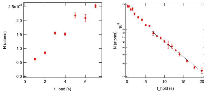
**Fig. 3.** (left part) Number of atoms in the MOT as a function of loading time; (right part) Number of remaining atoms in the MOT as function of the holding time; the line is a fit with a single exponential (see text). In both cases  $\Delta = -35\Gamma$  and total laser power on the ZS is 130 mW.
