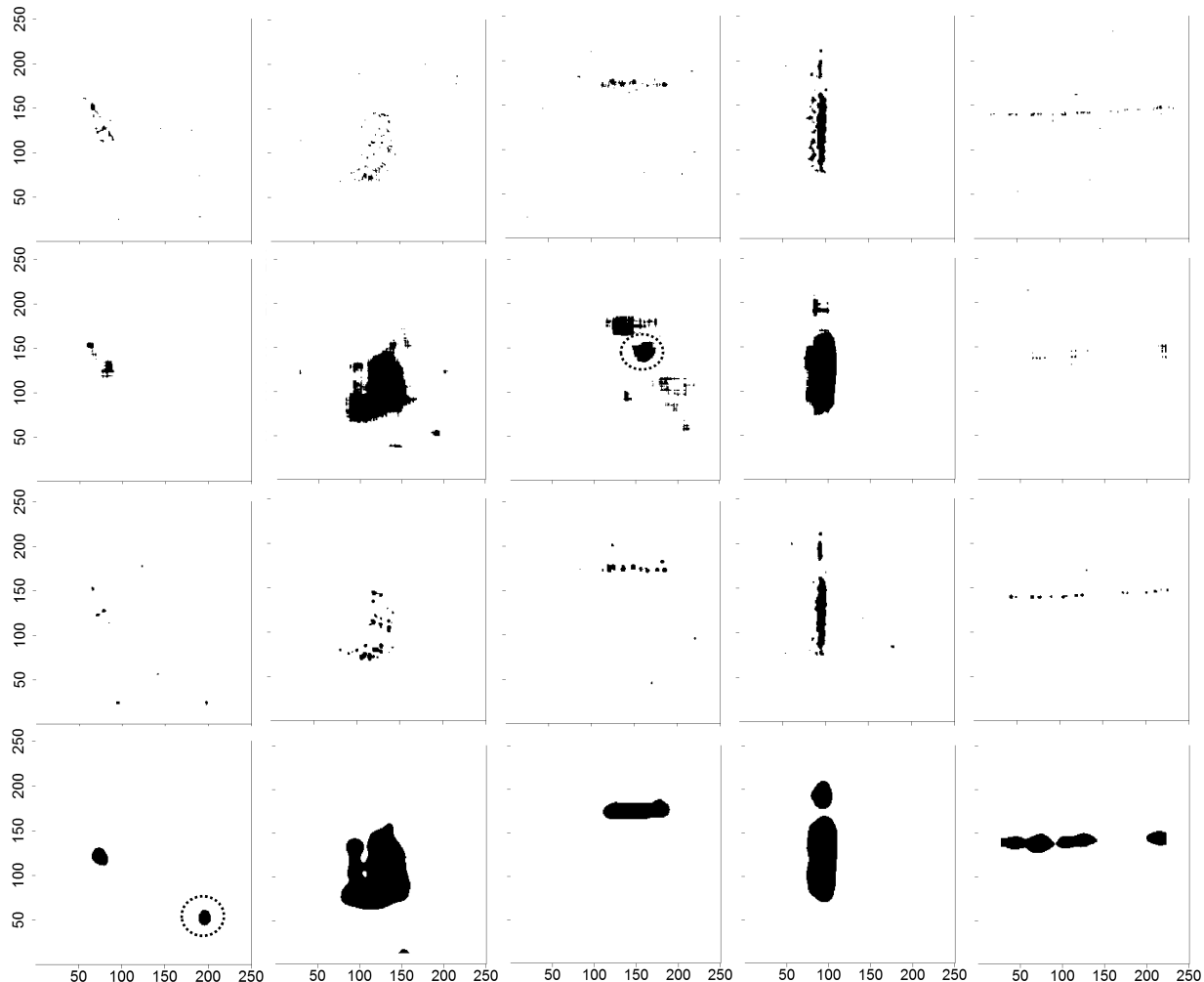
Figure 9. Diagnostic images of our algorithm for the defect-containing images in Figure 8 using: (1 st row) A-D-based statistic with w = 5 , (2 nd row) A-D-based statistic with w = 25 , (3 rd row) B-P-type statistic with w = 5 , and (4 th row) B-P-type statistic with w = 25 . In each row, the first—last columns correspond to Figures 8(a—e), respectively. The circled region is not a defect that we deliberately created, but it may indicate moderately abnormal local behavior in the fabric.
