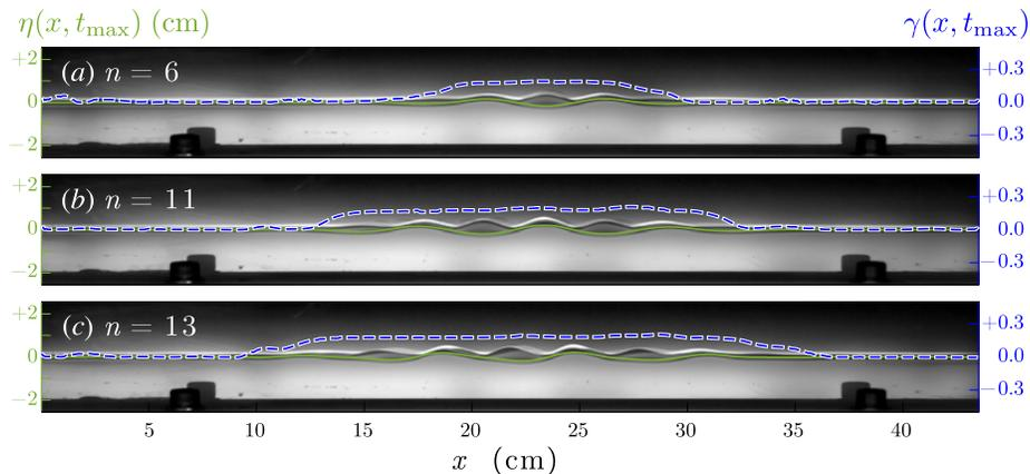
Figure 2. (Color online) Snapshots of the observed structures under localized forcing for different excitation regions: From top to bottom  $\sigma_i = 96, 176, 208$  mm. Green continuous lines depict the detected free-surface deformations at the wall, while blue dashed curves, the profiles of the effective acceleration at the surface.
