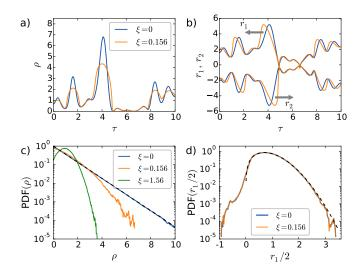
FIG. 1: Numerical simulation of Eq. (1) between  $\xi=0$  and  $\xi=0.156$  with  $\epsilon=0.014$ . Time evolution of (a)  $\rho$ , (b)  $r_{1,2}$  and (c), (d) associated PDFs. In (c) the black dashed line represents the exponential distribution  $\mathcal{P}(\rho)=e^{-\rho}$  and in (d), it represents the Rayleigh distribution  $(\mathcal{P}(x)=2xe^{-x^2/2})$ . The PDF in green line in (c) is obtained at  $\xi=1.56$  where the wave system has reached a statistical stationary state.
