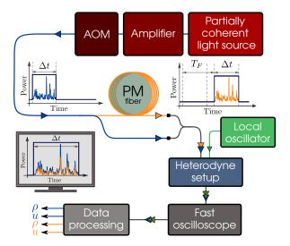
FIG. 2: Experimental setup. Partially coherent light at 1064 nm is injected inside a 1.4-km-long PM fiber in a regime where nonlinear effects strongly dominate linear ones ( $L_{NL}=1.3$  km,  $L_D=6250$  km,  $\epsilon=0.014$ ). Real-time observation of  $\rho(\tau)$  and of  $u(\tau)$  at the input and output ends of the PM fiber is achieved by combining a time-division multiplexing technique and an heterodyne measurement (see text).
