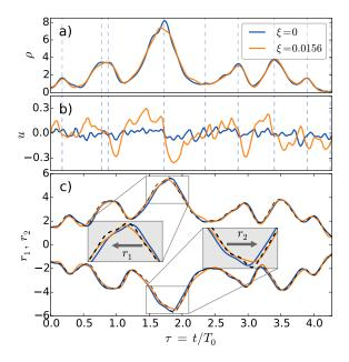
FIG. 3: Experiments. Time evolution of  $\rho$ , u, and of the Riemann invariants  $r_{1,2} = u \pm 2\sqrt{\rho}$  at the input end ( $\xi = 0$ ) and at the output end ( $\xi = 0.0156$ ) of the fiber ( $T_0 = 250$  ps). The black dashed lines represent Riemann invariants calculated from numerical integration of Eqs. (5) while starting from the experiment initial conditions (blue lines).
