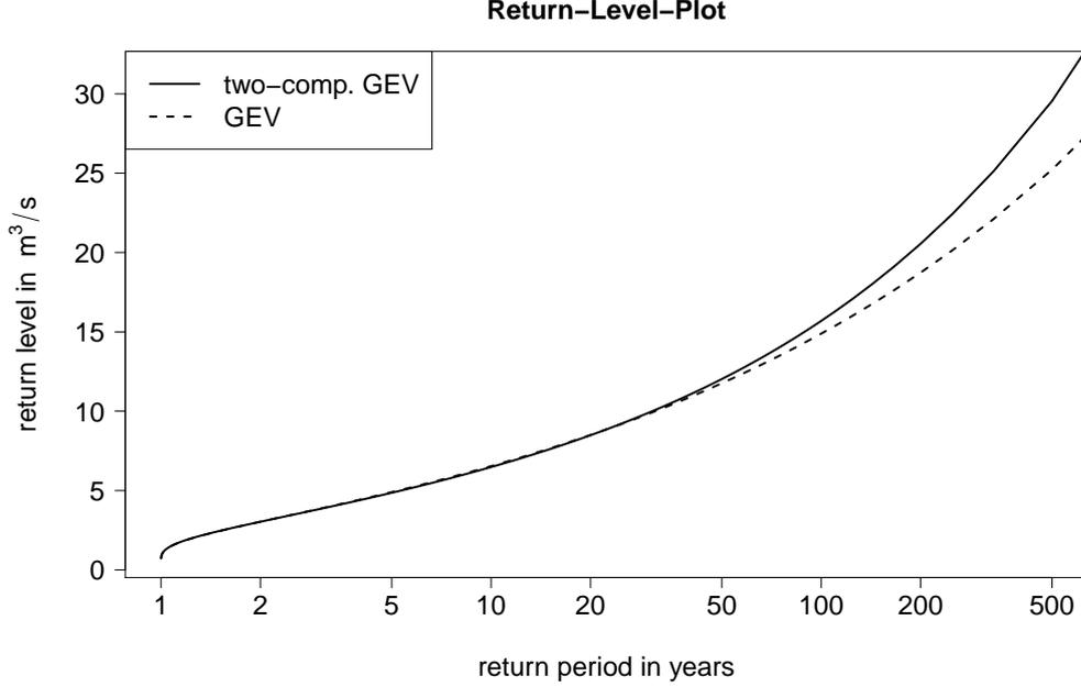
Figure 3: Return level plot of a two-component GEV  $F$  with  $\theta_w = (2, 1, 0.2)'$  and  $\theta_s = (1.5, 1, 0.4)'$ , and that of a GEV with  $\theta^* = (2.554, 1.235, 0.305)'$  minimizing the Kullback-Leibler distance to  $F$ .
