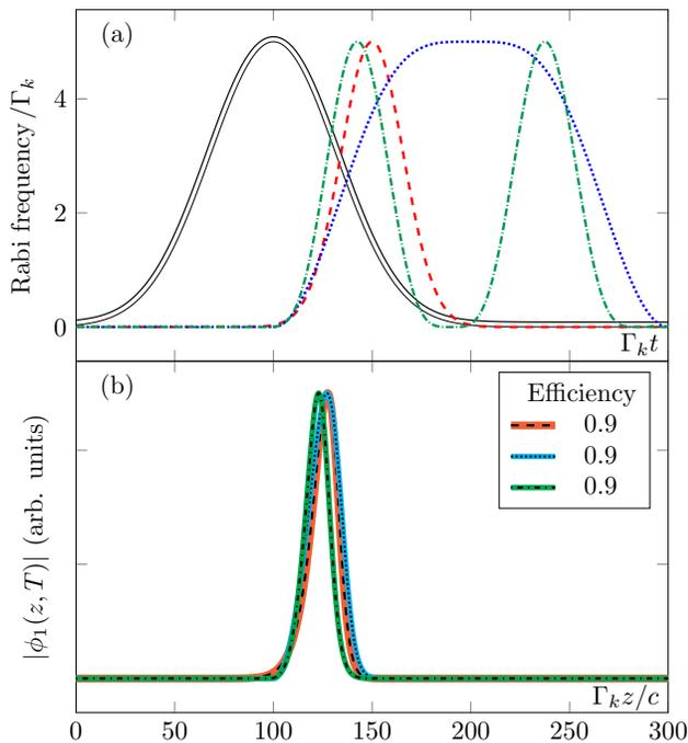
FIG. 2: (a) Various pulse shapes of the pump  $\Omega_p(t)$  (dotted, dashed and dash-dotted lines) with the maximum value  $\Omega_{p\max} = 5\Gamma_k$  and the shape of the emitter-cavity interaction  $g(t)$  (double line, shown as normalized to  $\Omega_{p\max}$ ). (b) Corresponding spatiotemporal shapes of the one-photon Fock state outgoing wave packet ( $R_k = 5\Gamma_k$ ,  $\Delta_k = \Delta_p = \Gamma_k$ ,  $T = 350\Gamma_k$ ).
