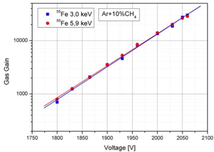
Figure 45: The gain versus the high voltage at the divider is shown for P10 construction using the scalable readout system and the APV25 hybrids.
