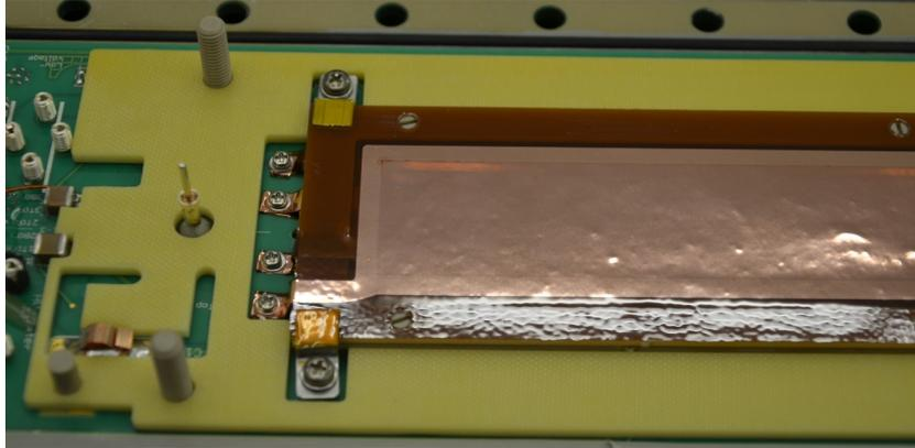
Figure 56: Picture of a GEM-stack screwed to the pad-plane.
