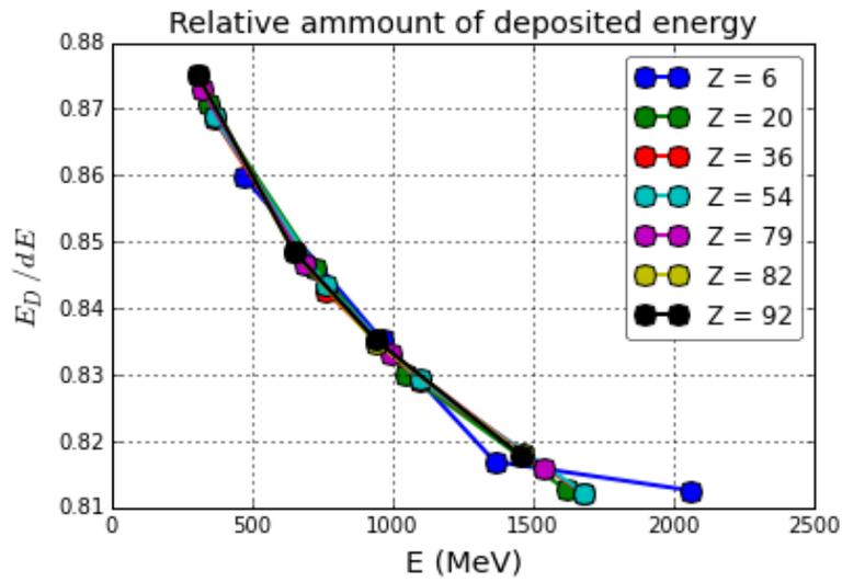
Figure 70: Calculated relative deposited energy in HGB4 as a function of energy and charge of the projectiles.
