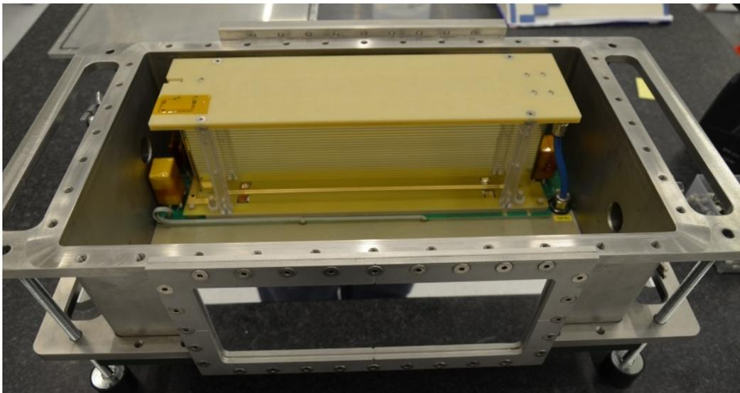
Figure 31: Picture of the first of two compartments of HGB4 installed inside the stainless steel vessel.
