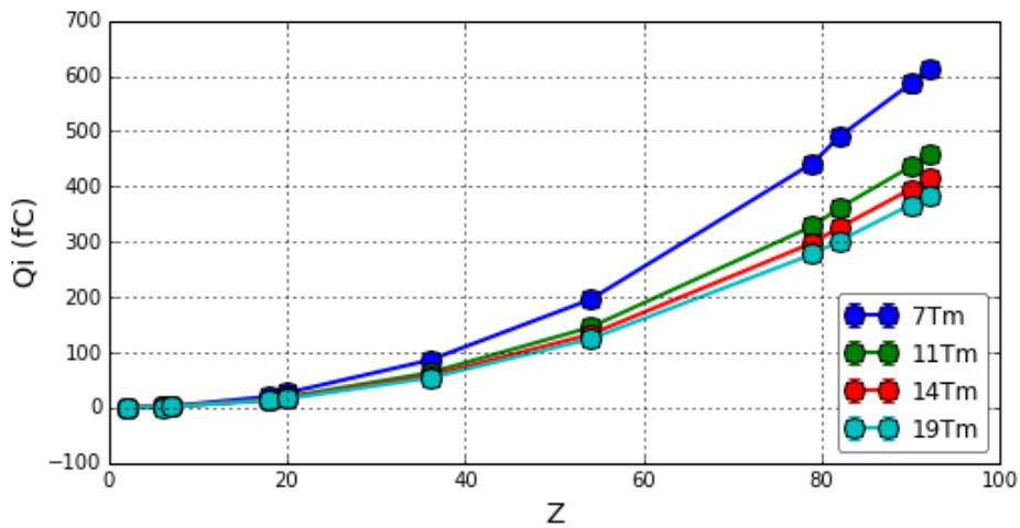
Figure 71: The charge deposited in the active volume of HGB4 for different ions and  $B\rho$ .
