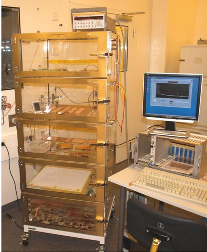
Figure 38: Leakage current measurement set-up.
