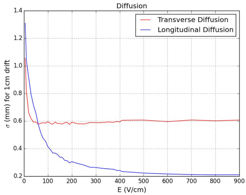
Figure 23: Longitudinal and transverse diffusion of electrons in a P10 gas mixture as a function of the applied electrical field.
