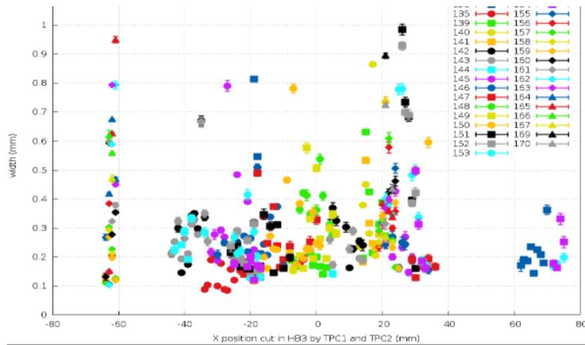
Figure 75: Measured horizontal position resolution of the GEM-TPC prototype (no twin) for different runs, corresponding to different beam positions.
