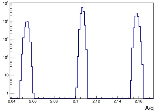
Figure 65:  $A/Q$  distributions of  $^{37-39}\text{Ar}$  at about 1.4 GeV/u assuming 0.5 mm TPC resolution and 20 ps TOF resolution at FHF1 distance of about 1 m.
