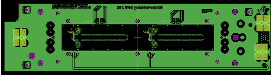
Figure 50: Snap shot of the back-side of the pad-plane of HGB4. The 512 electrodes on the front-surface are internally routed to two SAMTEC 300-pin high-density connectors each connecting 256 pads.
