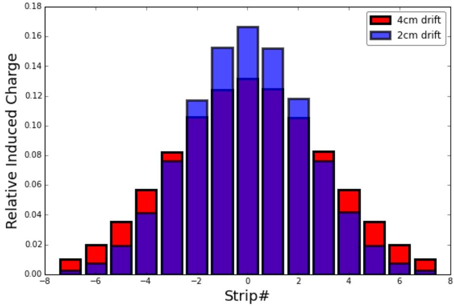
Figure 72: Relative induced charge on the pad-plane. The red and blue histograms corresponds to the 4 and 2 cm drift lengths, respectively.
