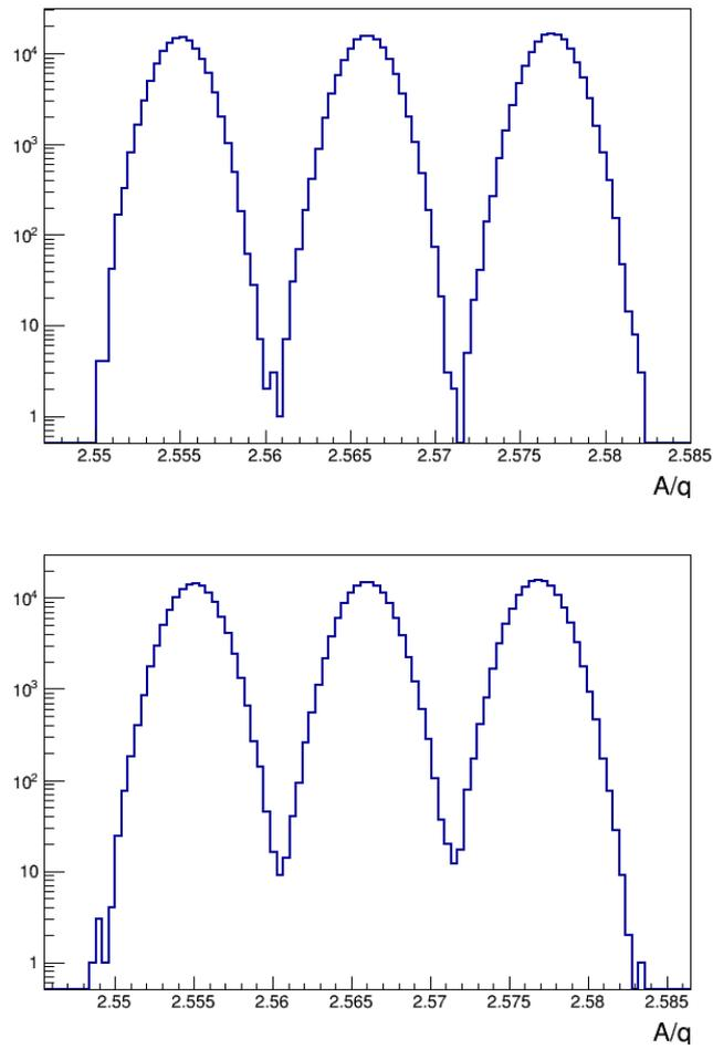
Figure 64:  $A/Q$  distributions of  $^{235-237}\text{U}$  at about 1.4 GeV/u assuming 0.5 mm TPC resolution and 20 ps TOF resolution. Top: HFH1 distance equal to about 1 m, Bottom: HFH1 distance equal to about 7 m
