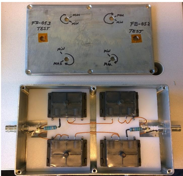
Figure 34: Field cage resistor terminator.
