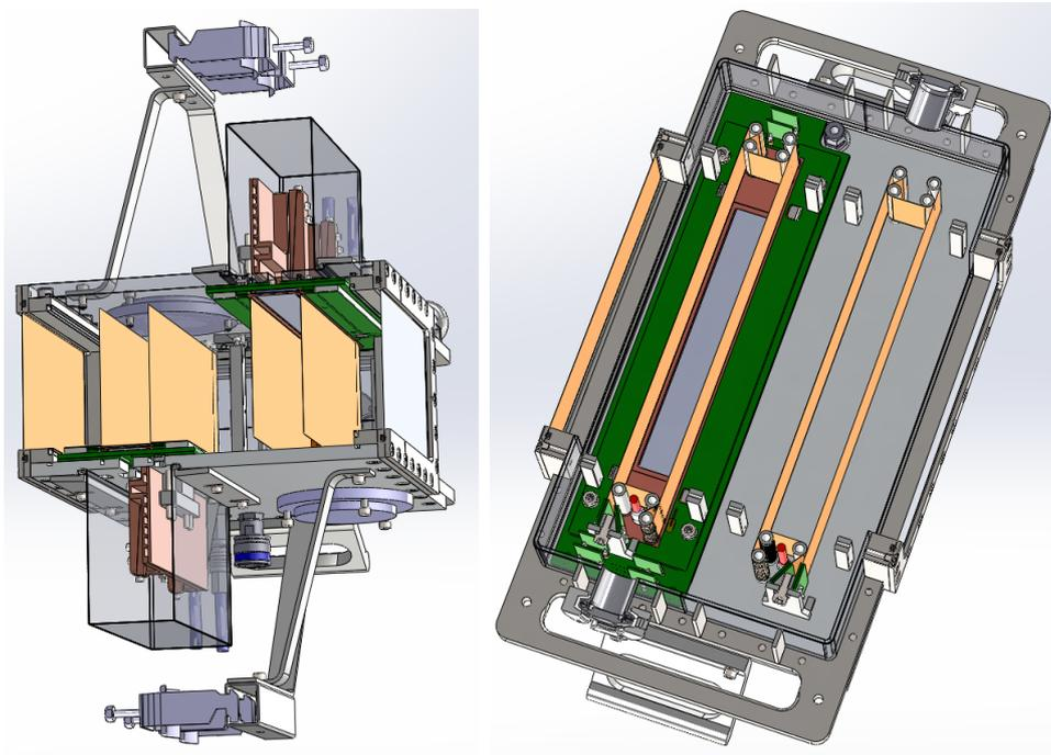
Figure 9: CAD sketch of the field-cage compartments of HGB4 demonstrating their arrangement and the various thin layers of material the beam has to pass (horizontally from left to right).
