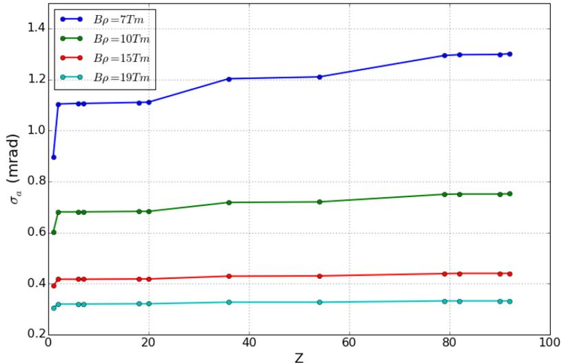
Figure 69: Calculated angular straggling due to the whole HGB4 matter.
