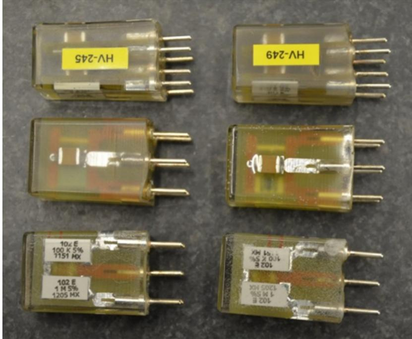
Figure 52: Picture of two complete sets of high-voltage filters employed to filter the bias voltages for the GEM-foils.
