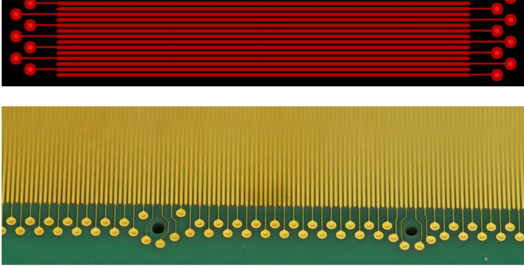
Figure 48: CAD design (upper part) and snap shot (lower part) of the surface of pad-plane of HGB4 facing the gas volume. The inner active area is patterned with 512 strip-type electrodes of 30 mm in length and 0.25 mm in width, the gap between neighbouring pads is 0.15 mm and the pitch is 0.4 mm.
