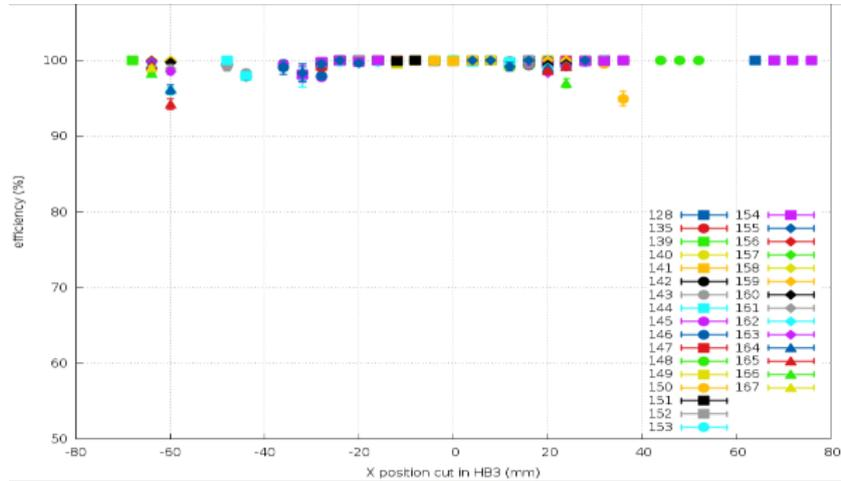
Figure 76: Measured efficiency of the GEM-TPC prototype (HB3) (no twin) for different runs, corresponding to different beam positions.
