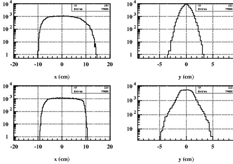
Figure 2: Horizontal and vertical distributions at FPF2 (dispersive focus) in front (upper panels) and behind (lower panels) the focus.
