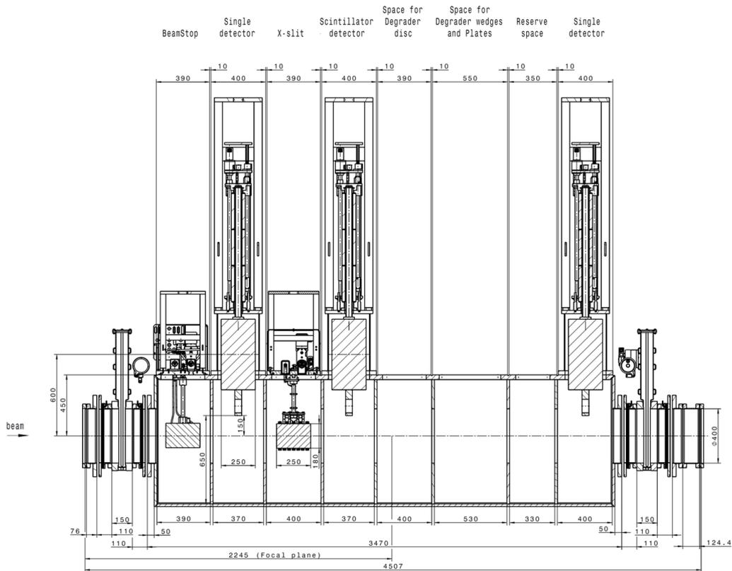
Figure 20: Super-FRS diagnostic chamber at FPF2.
