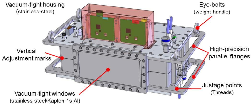
Figure 14: CAD sketch of the chamber housing emphasizing various design details which support the adjustment during mounting.
