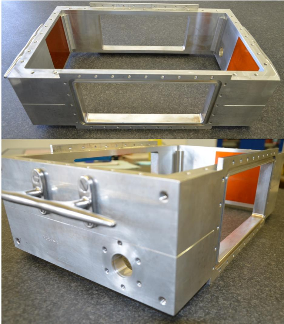
Figure 11: Housing milled-out from a single block of Aluminium.
