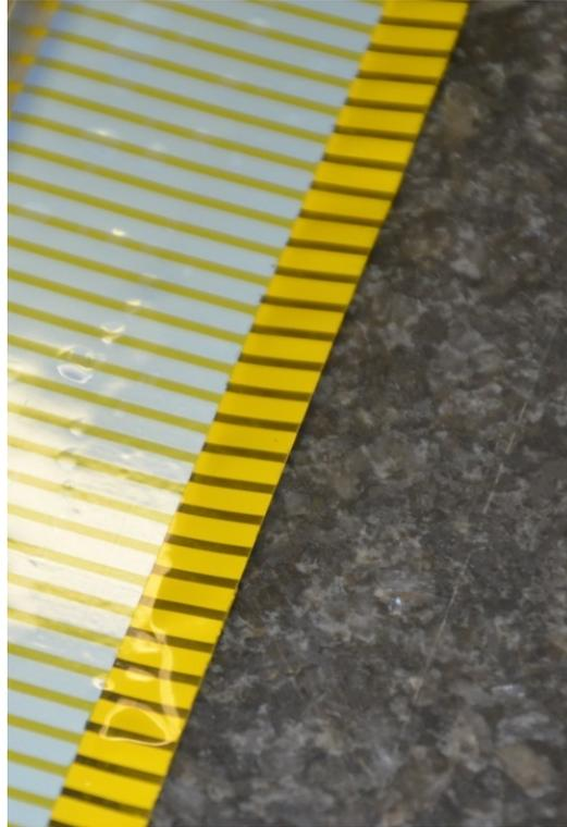
Figure 26: Picture of the field-cage strip-line foil, the staggered structure of the field defining aluminium stripes in the front as well as the mirror stripes on the back-side surface are clearly visible.
