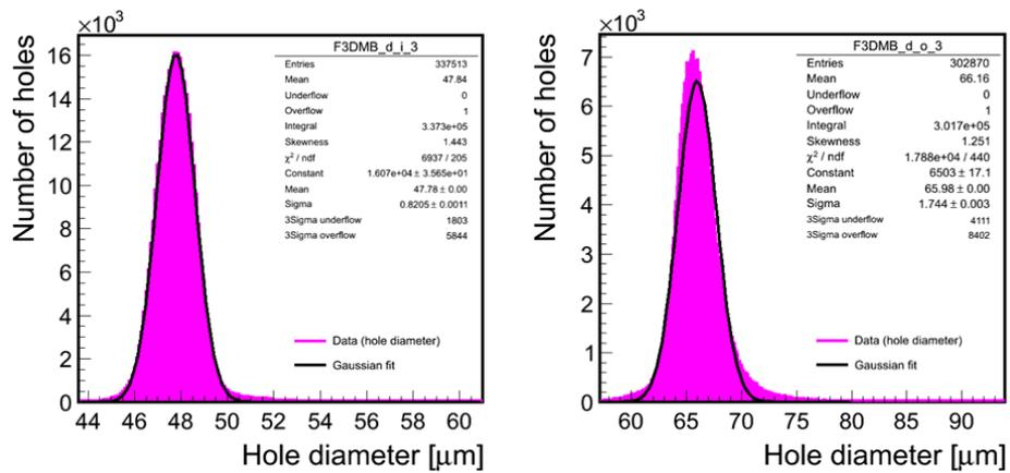
Figure 42: Distribution of the hole diameter for the HGB4 foil. The inner and outer hole diameters are shown on the left and right correspondingly.
