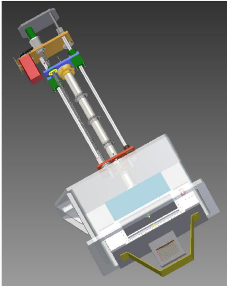
Figure 21: HGB4 attached on to the ladder arm. The SEM-Grid beam profile monitor is attached on the bottom flange of HGB4.
