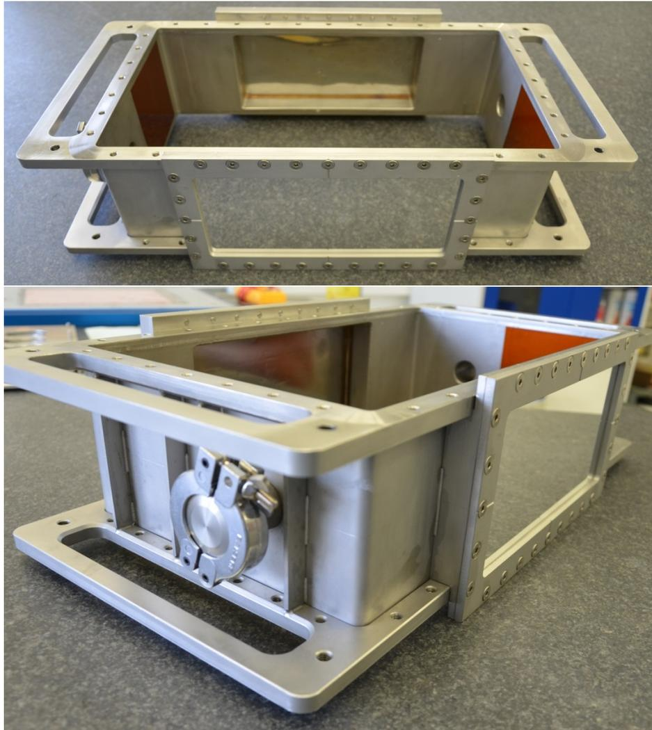
Figure 10: Housing made from stainless steel in a welding-type construction. The KF-type exhausts can be used to evacuate the vessel enforcing out-gassing of the detector materials installed inside in order to achieve better gas-purity.
