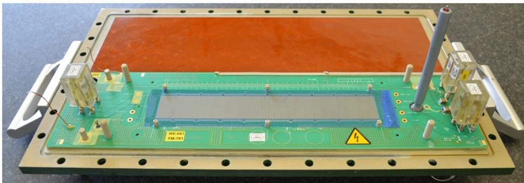
Figure 46: Picture of the actual pad-plane mounted on one of the panel flanges of HGB4.
