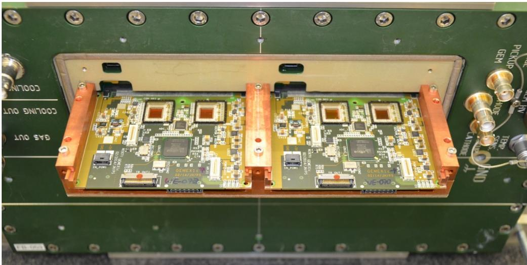
Figure 19: The active copper cooler with the cover heat-screen removed and the actual GEMEX1C read-out boards installed (the interlinking GEMCON PCB bridge has also been removed).
