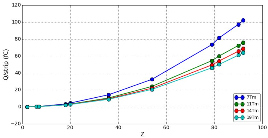
Figure 73: Maximum induced charge per strip for different fragments and  $B\rho$ .
