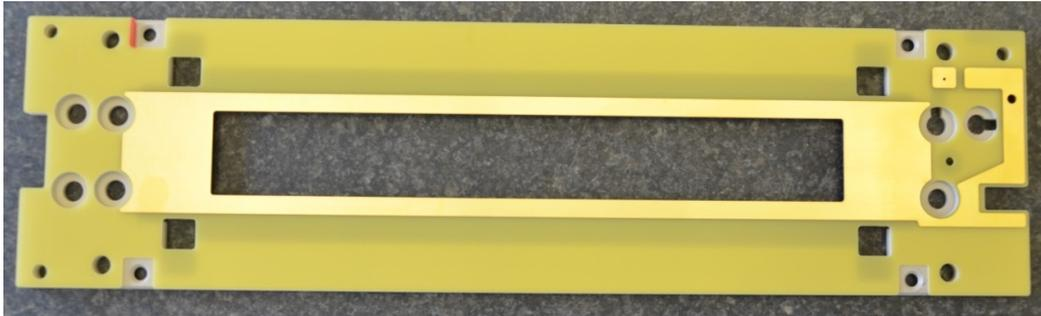
Figure 25: Picture of the field-terminating plate mounted on its backing.
