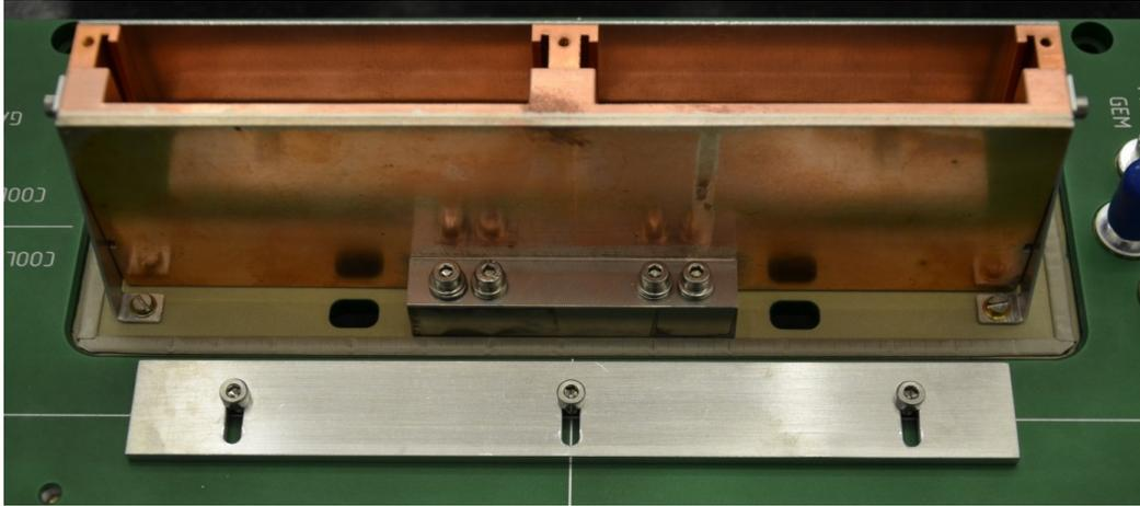
Figure 18: The active copper cooler.
