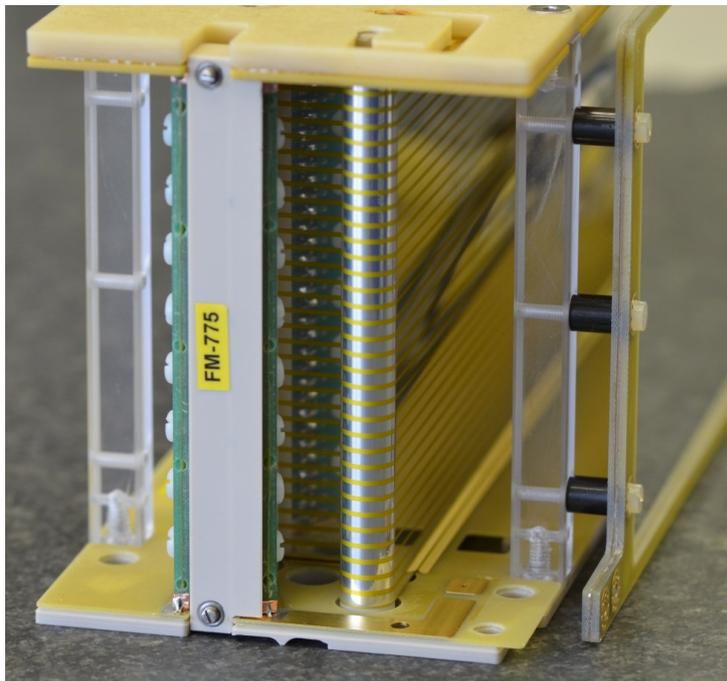
Figure 29: Picture of one of the two field-cages of HGB4. Two identical resistor dividers operated in parallel are mounted on both ends of the strip-line type field-cage foil. The double-sided metallized foil mounted in between the two field cage compartments of HGB4 for screening purpose is also visible.
