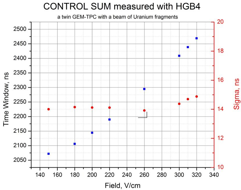
Figure 77: The control sum scan at different fields; from 150 V/cm up to 320 V/cm. In blue the total sum and in red the time resolution.
