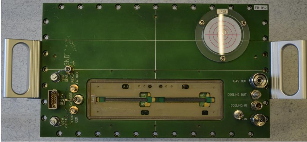
Figure 12: Overview picture of one of the back-side of the flanges mounted to HGB4 facing the inside volume of the detector. The two groups of grooves as part of the distribution of the fluidal supplies are visible as well as the screw-mounted connectors
