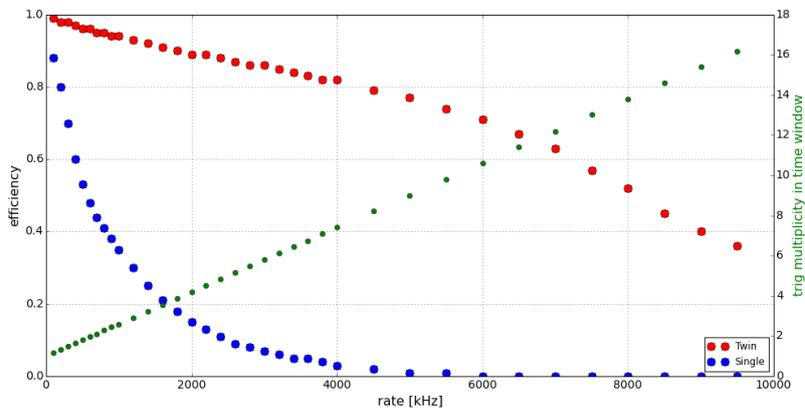
Figure 74: Simulated efficiency for HGB4 twin design (red) and single volume detector (blue) as a function of rate. The green points represent the mean number of hits in collection time at given rate (scale on the right axis).
