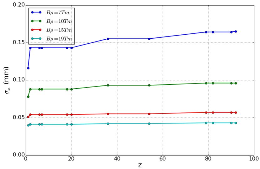
Figure 68: Calculated position straggling in the middle of the HGB4 detector.
