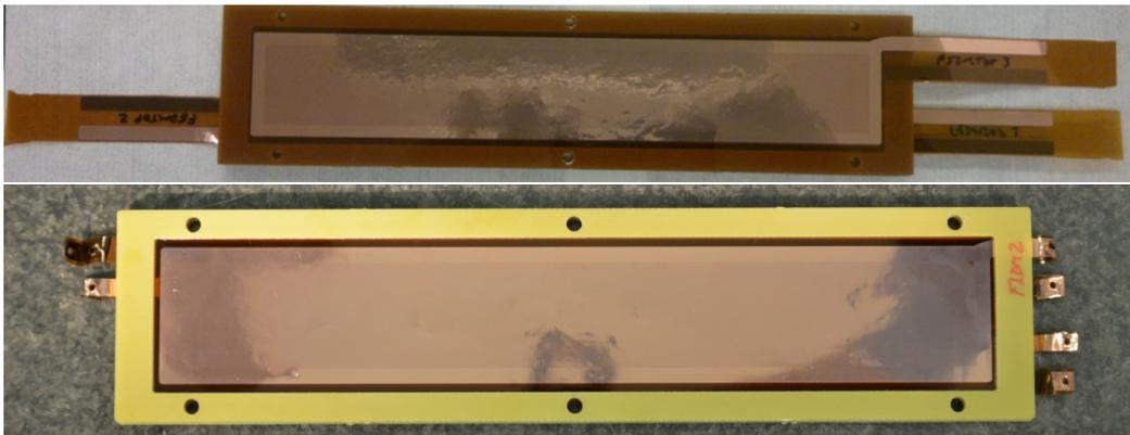
Figure 55: Picture of a set of three framed GEM-foils forming the amplification stage of a single compartment of HGB4 from the top side with uncut flaps (upper part) and from the bottom side with cut flaps 'ready-to-mount' (lower part).
