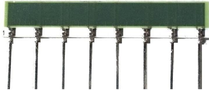
Figure 36: GEM stack passive divider.
