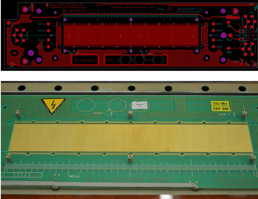
Figure 47: CAD design (upper part) and snap shot (lower part) of the surface of pad-plane of HGB4 facing the gas volume. The inner active area is patterned with 512 strip-type electrodes.
