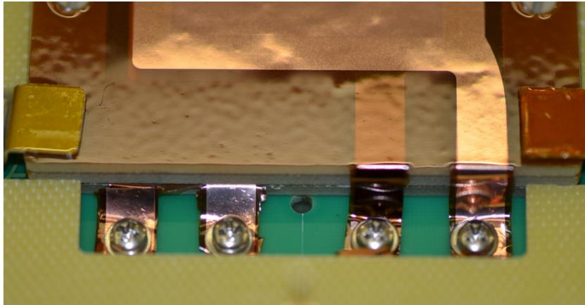
Figure 57: Picture of the flaps of the GEM-stack screwed to the pad-plane.
