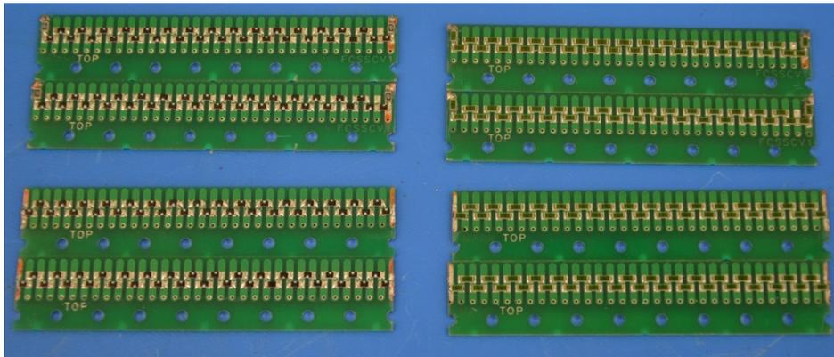
Figure 27: Picture of the resistor dividers for two identical field-cages in HGB4. The left part shows the PCB with standard resistors part-mounted, the right pair is equipped with high-precision high-voltage type SMD resistors.
