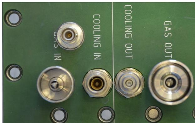
Figure 17: Picture of the fluidal supplies, the detector gas as well as the cooling fluid. Note that it has been decided only after the flanges have already been produced to provide the first strip of the field cage with autonomous biasing.
