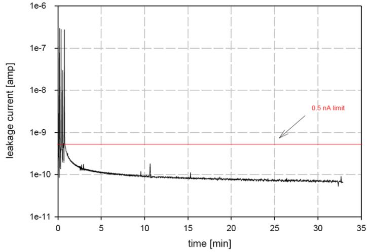
Figure 39: Leakage current resulting from a good working GEM foil. The evolution of this step in the characterization shows that the GEM foil performs well and it is accepted. The acceptance criteria is a leakage current of less than 0.5 nA for 30 min at 500 V in dry atmosphere.
