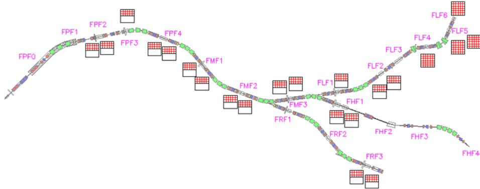
Figure 1: Layout of Super-FRS and the tracking detectors (red symbols). At all focal planes, except FLF4, FLF5 and FLF6, each tracking detector is integrated in a ladder.
