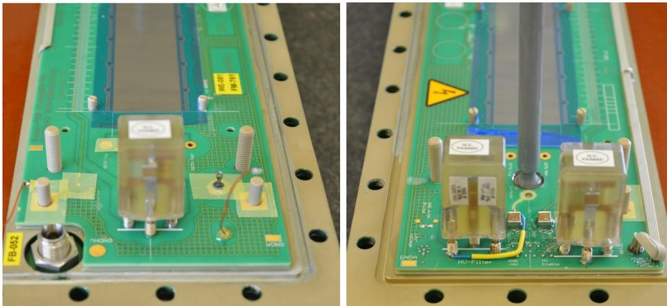
Figure 53: Picture of two complete sets of high-voltage filters employed in order to filter the bias voltages for the GEM-foils.
