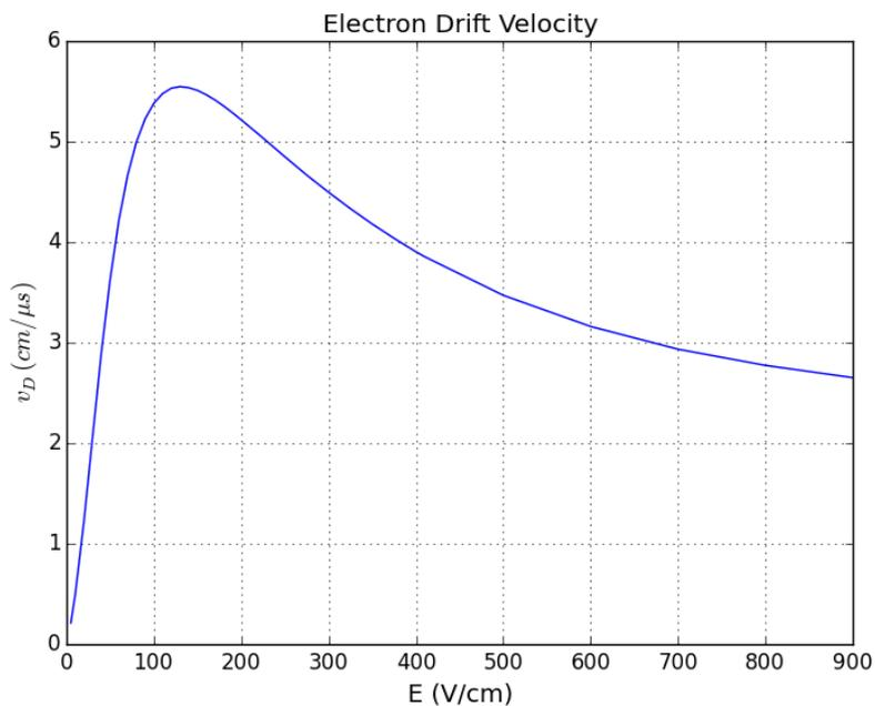
Figure 22: Electron drift velocity in a P10 gas mixture as a function of the applied electrical field.
