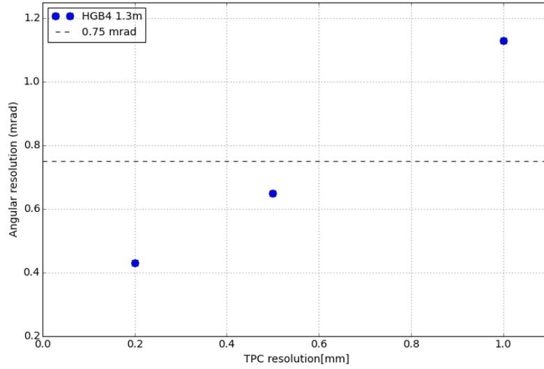
Figure 67: The calculated FHF1 angular resolutions of  $^{236}\text{U}$  for 1 m distance as a function of the position resolution.
