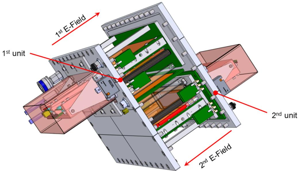
Figure 8: CAD sketch of the field-cage compartments of HGB4.
