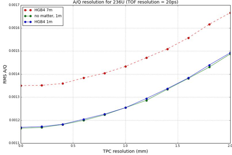
Figure 63:  $A/Q$  resolution of  $^{236}\text{U}$  fragments at about 1.4 GeV/u as a function of TPC position resolution. The TOF resolution of 20 ps is assumed.
