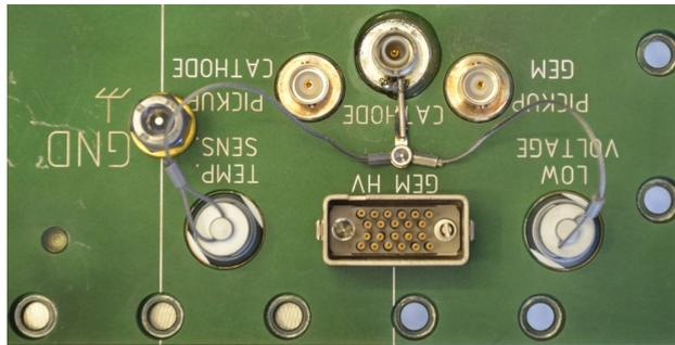
Figure 16: Picture of the electrical supplies and signals: Ground (GND), low, high, and bias voltages, sensor and pick-up signals.
