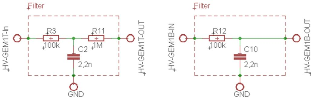
Figure 51: Electrical schematics used for the HV filters here exemplary showing connections to the top (T) and bottom (B) surfaces of GEM no. 1.
