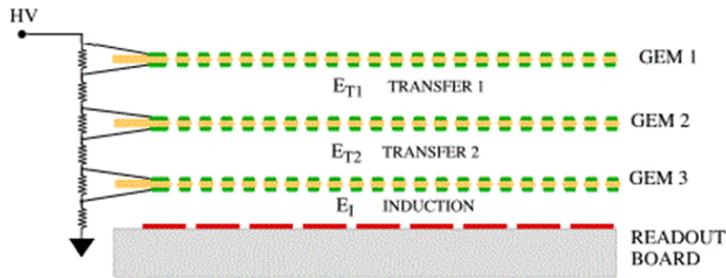
Figure 35: GEM stack power scheme.
