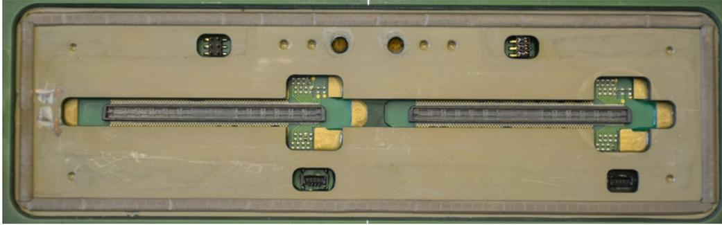
Figure 54: Picture of two adjacent high-density read-out connectors mounted on the back-side of the Pad-plane PCB (the copper cooler has been removed for that purpose).
