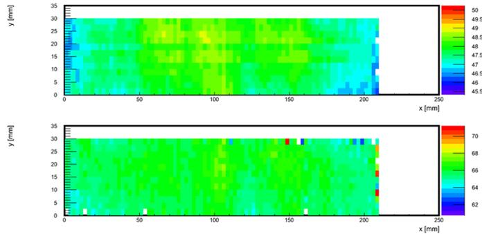
Figure 43: Map for the distribution of the hole diameter for the HGB4 foil. The inner and outer hole diameters are shown on the top and bottom panels, correspondingly.
