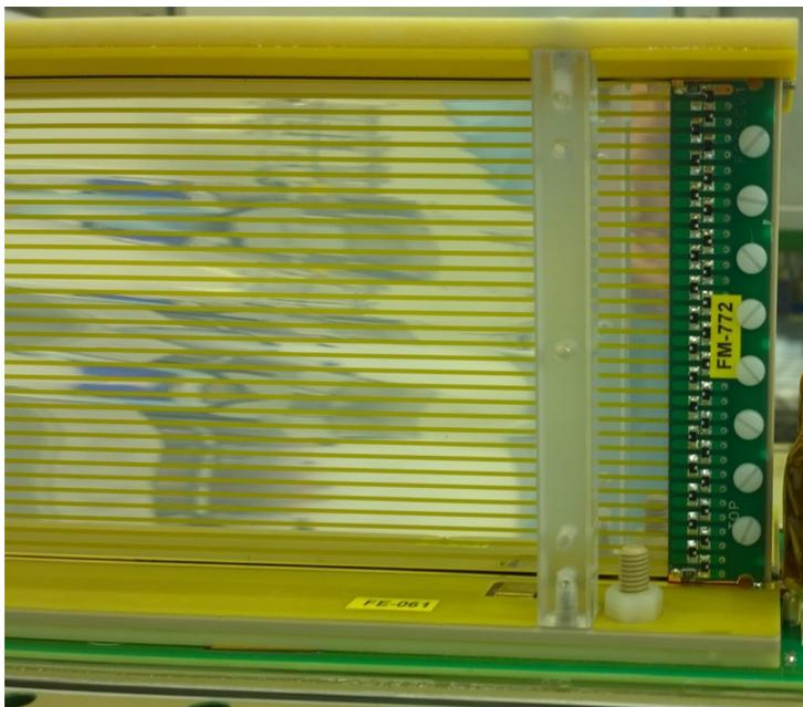
Figure 33: Field cage resistor divider.
