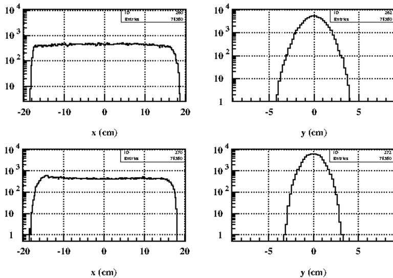
Figure 5: Horizontal and vertical distributions at FMF1/FMF3 in front (upper panels) and behind (lower panels) the focus.
