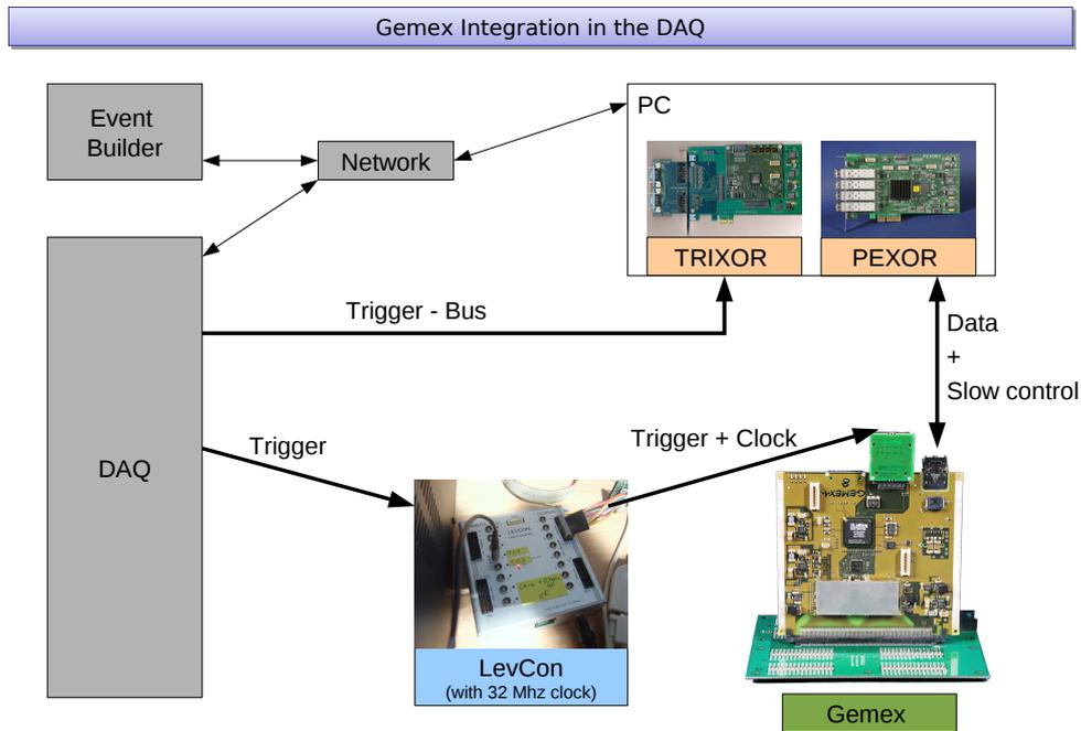
Figure 60: Integration of the GEMEX card into the MBS DAQ [15] .
