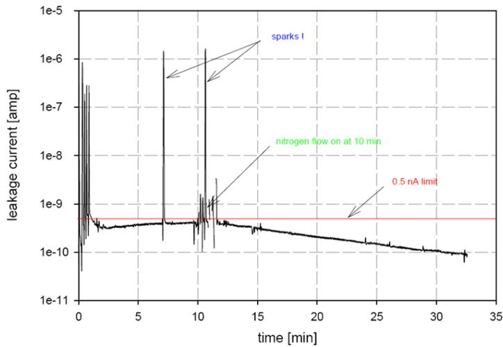
Figure 40: Leakage current resulting from a recovered GEM foil
