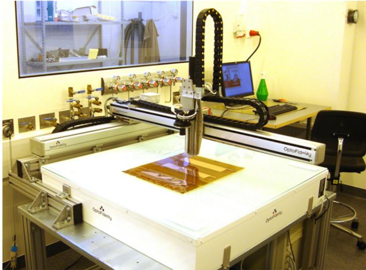
Figure 41: Set-up of the high-resolution scanning system.
