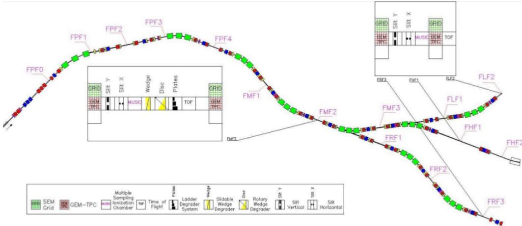
Figure 62: Layout of Super-FRS and the standard detector configuration at FMF2, FLF2, FHF1 and FRF3.
