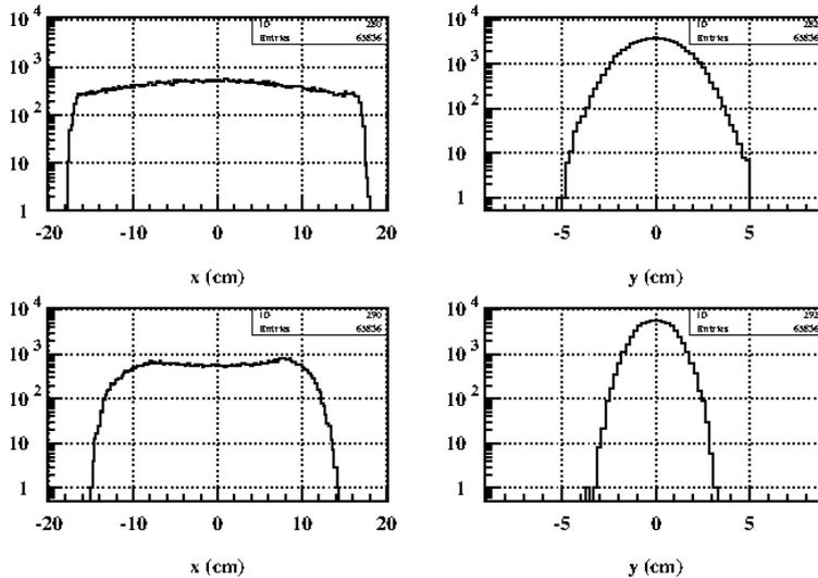
Figure 6: Horizontal and vertical distributions at FMF2 (achromatic focus) in front (upper panels) and behind (lower panels) the focus.
