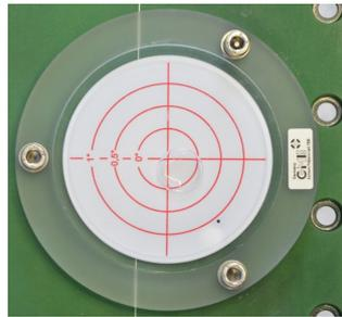
Figure 15: Picture of the bubble-level device mounted on the detector flanges allowing a horizontal adjustment of the detector.
