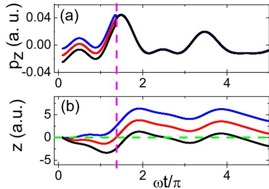
FIG. 3: (Color online) The evolution of the electron trajectories originating near the saddle point: (a) the evolution of  $p_z$ . (b) the motion along the laser propagation direction. The vertical dashed purple line throughout (a)(b) indicates the moment when the electron returns, i.e.,  $x(\eta_r) = 0$ .
