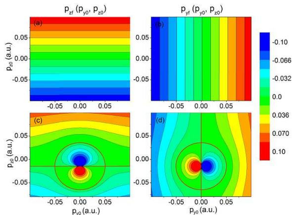
FIG. 2: (Color online) Contour plots of the asymptotic momentum  $P_{zf}$  (a and c) and  $P_{yf}$  (b and d) versus the initial transverse momentum at a fixed tunneled phase  $\omega t_0 = 0.3$  for 3400 nm LP field. Panels (a) and (b) are without Coulomb potential while panels (c) and (d) are with Coulomb potential.
