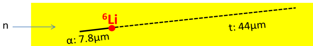
Fig. 1. After the absorption of neutron by {}^6\text{Li} loaded in nuclear emulsion, an alpha particle and a triton are emitted. A back-to-back topology is formed by their tracks. In the case of our fine-grained nuclear emulsion with \text{LiNO}_3 added, length of tracks of the alpha particle and the triton are 7.8 \mu\text{m} and 44 \mu\text{m} respectively from calculation by SRIM.
