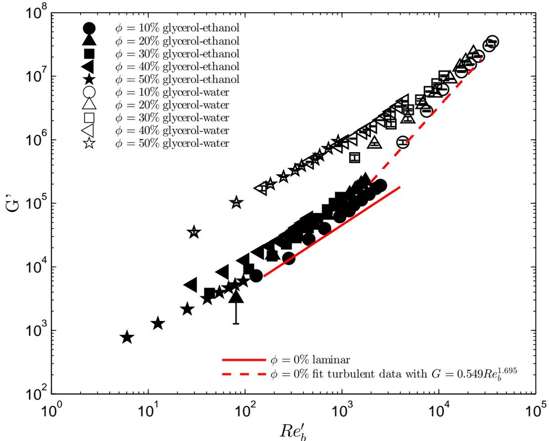
FIG. 10: Normalized torque measurements for all of the current experimental measurements,  $G'$  as a function of  $Re'_b$  using an effective viscosity model.
