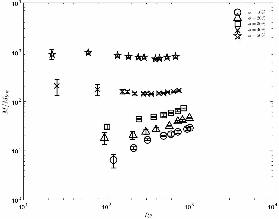
FIG. 6: Normalized torque as a function of Reynolds number for polystyrene particles immersed in the glycerol-water solution (low-viscosity fluid.)
