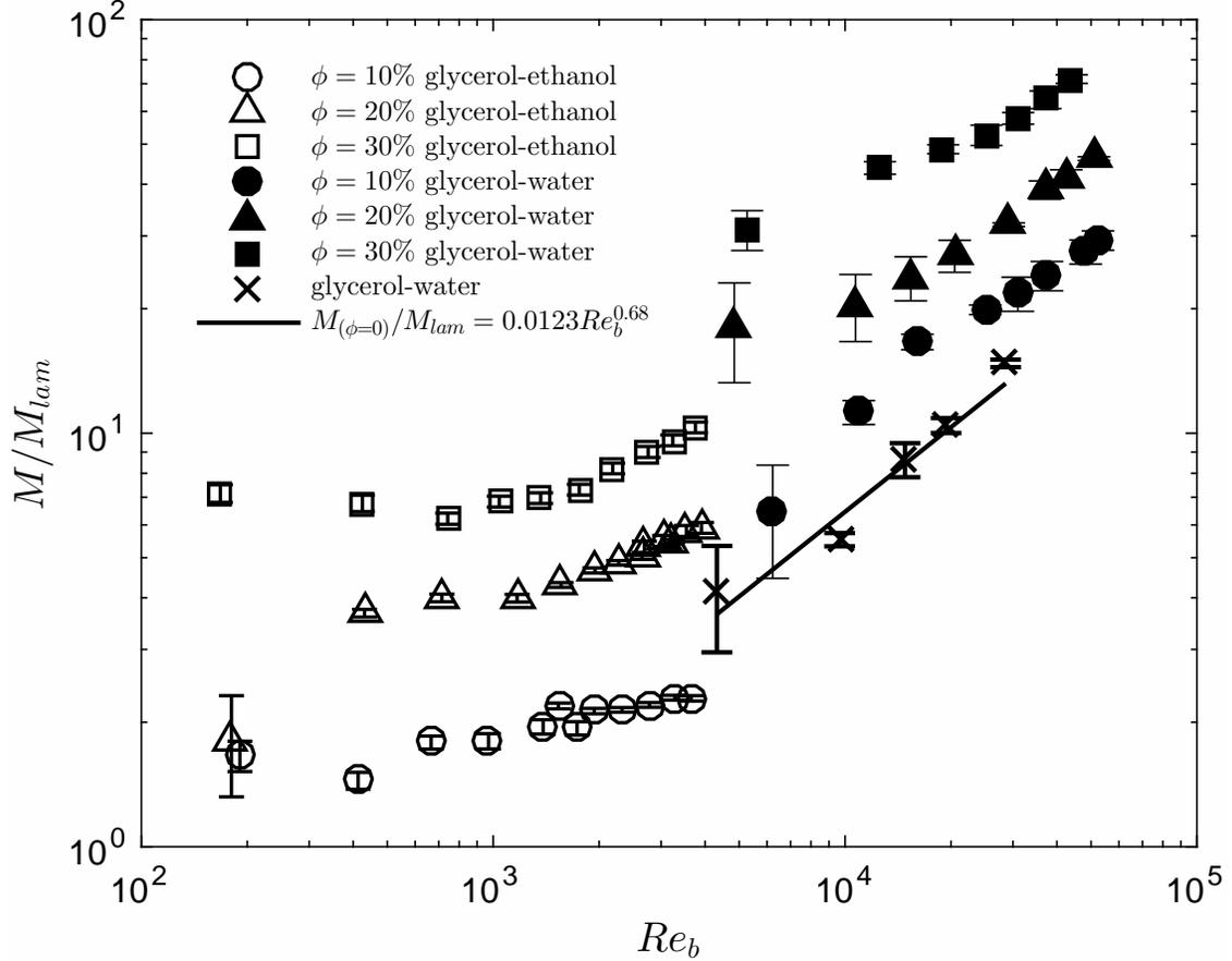
FIG. 7: Normalized torque as a function of gap Reynolds number for polystyrene particles immersed in the high- and low-viscosity fluids, respectively.
