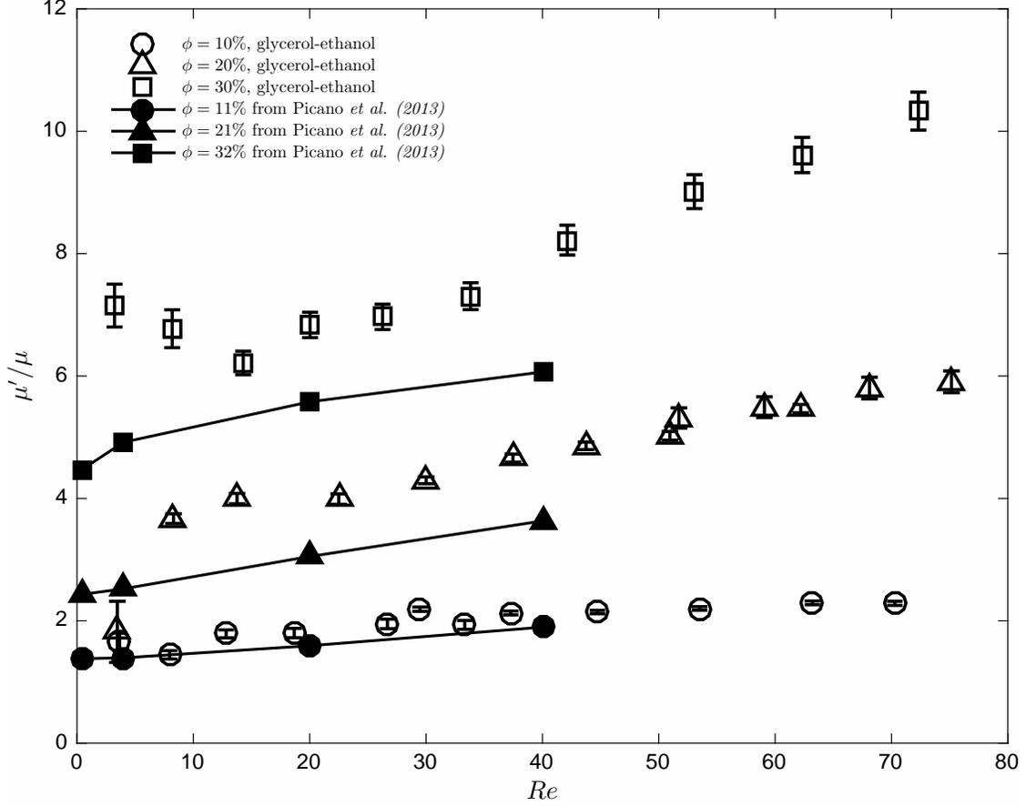
FIG. 5: Normalized torque (experiments) and effective viscosity (numerical results) as a function of Reynolds number. The experiments correspond to the polystyrene particles immersed in a high-viscosity fluid for  $\phi = 0.1, 0.2,$  and  $0.3$ . The simulations results are from Picano *et al.* [9].
