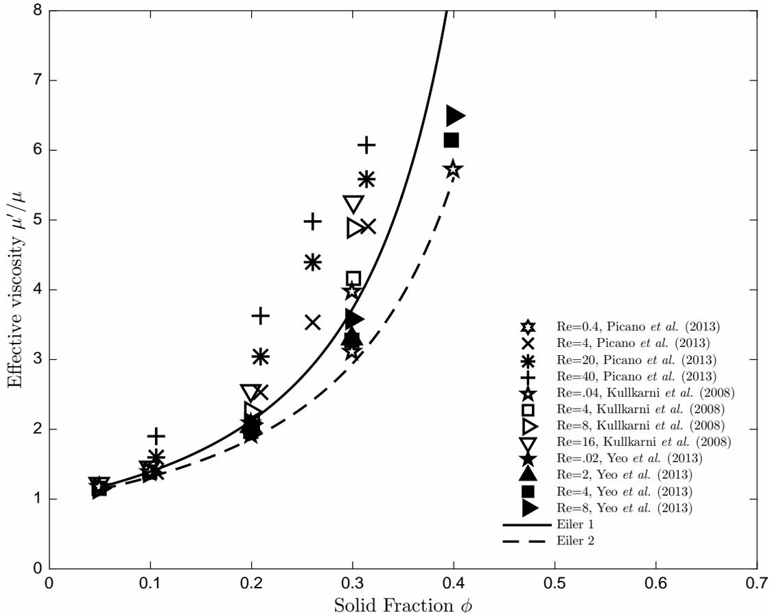
FIG. 1: Effective viscosity for inertial suspensions as a function of solid fraction from numerical simulations made by Kulkarni and Morris [6], Yeo and Maxey [8], Picano *et al.* [9]. Continuous and dashed lines correspond to Eilers relation with  $a = 1.5$  and  $\phi_m = 0.58$  and  $a = 1.25$  and  $\phi_m = 0.63$  respectively.
