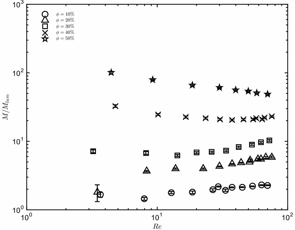
FIG. 4: Measured torque normalized by the theoretical pure fluid torque considering laminar flow, as a function of Reynolds number for polystyrene particles immersed in a glycerol-ethanol solution (high viscosity fluid.)
