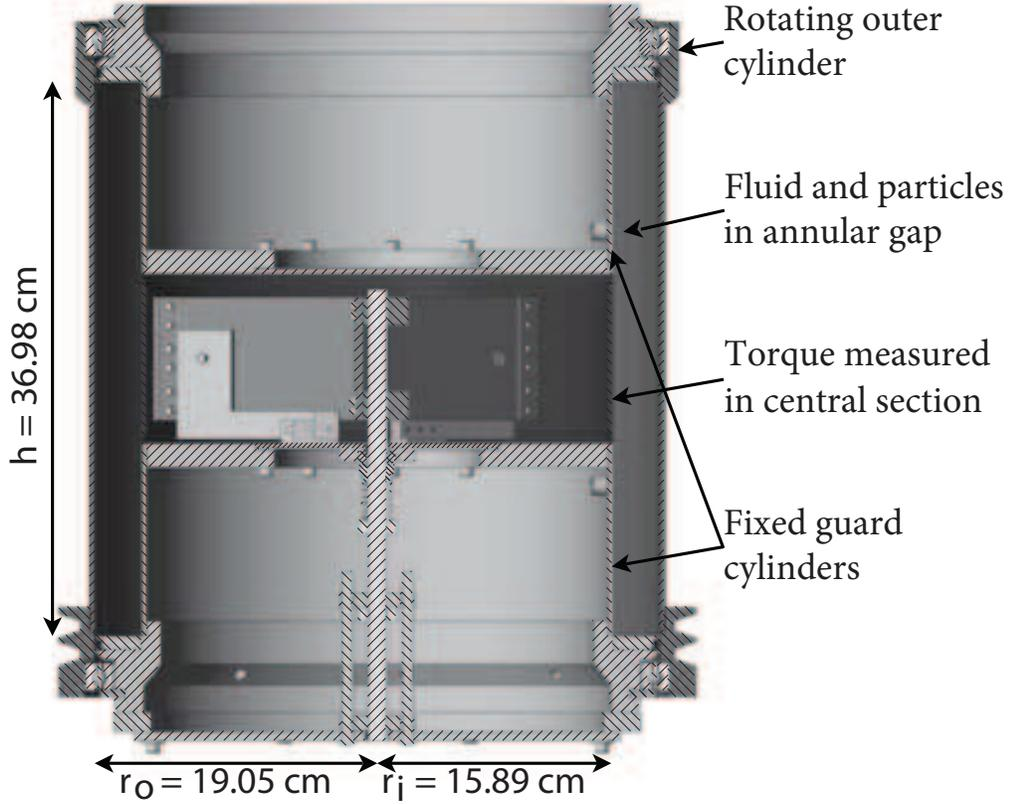
FIG. 2: Schematic of the coaxial cylinder rheometer.
