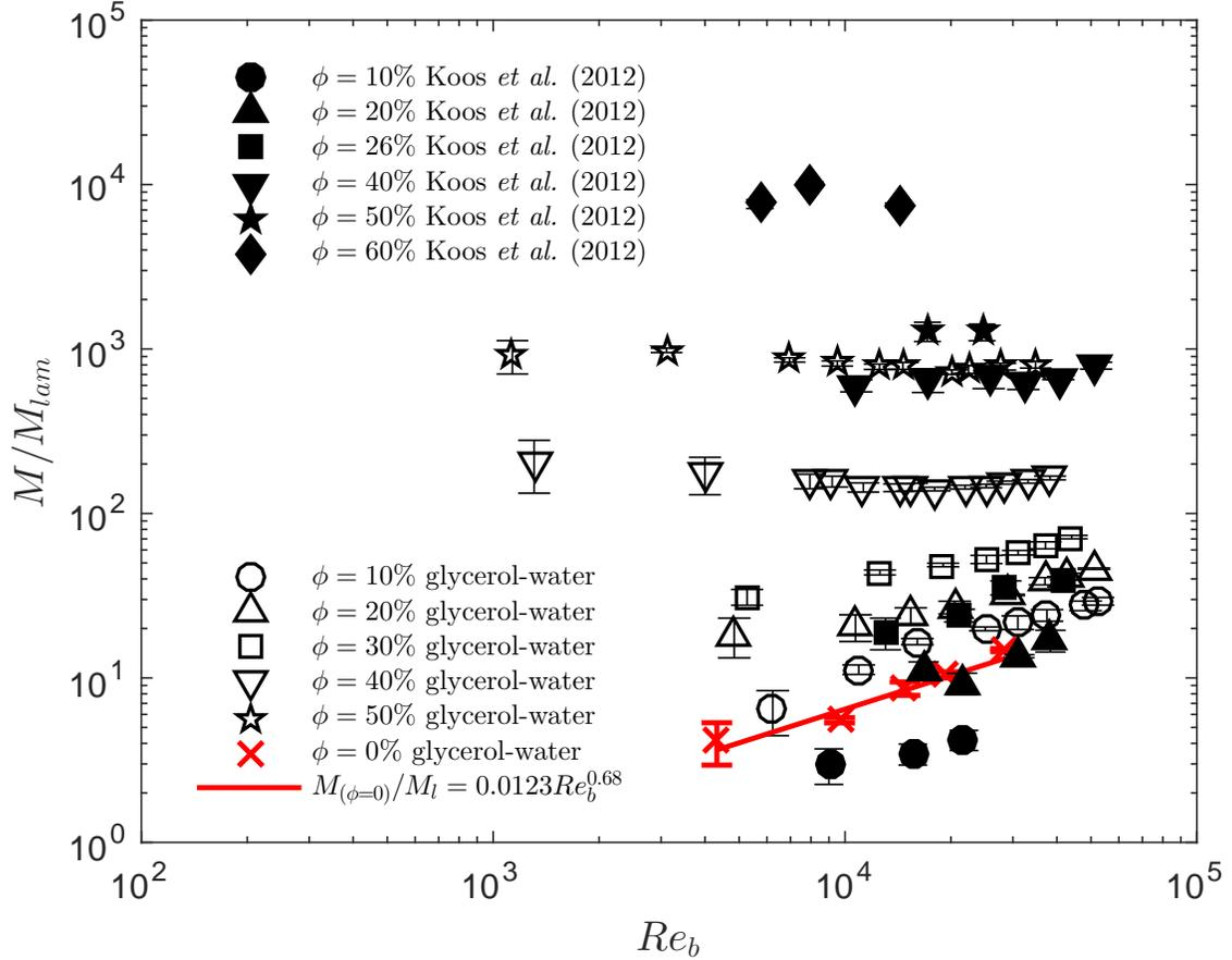
FIG. 9: Comparison between the normalized torques for the low-viscosity fluid and the results from Koos *et al.* [29] for rough walls experiments.
