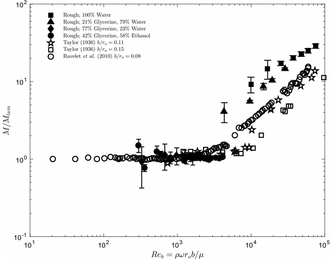
FIG. 3: Measured torque normalized by the theoretical pure fluid torque considering laminar flow, as a function of gap Reynolds number for different fluids. Open symbols correspond to the data from Taylor [32] and Ravelet *et al.* [39].
