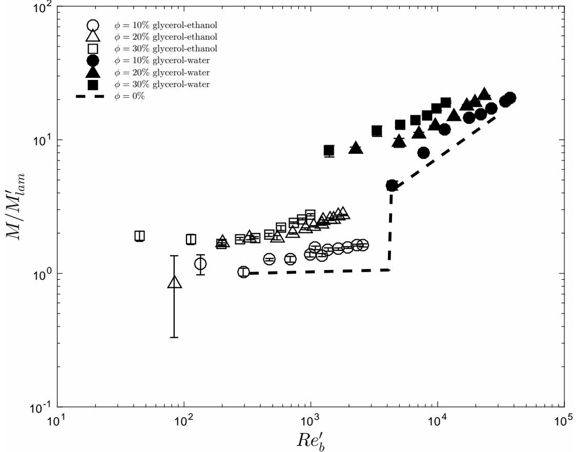
FIG. 8: Measured torque normalized by effective laminar torque (using the effective viscosity from the Krieger-Dougherty relation) as a function of effective gap Reynolds number for polystyrene particles immersed in the high- and low-viscosity fluids, respectively.
